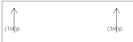
Figure 6-6: Equivalent nodal forces using the lumped approach.
