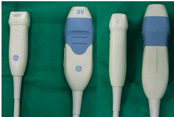
Fig. 23.1. Two ultrasound probes viewed from a frontal and lateral perspective. To the left of both panels an ordinary 2D phased array is shown and to the right in both panels a matrix probe, which enables real-time 3D ultrasound scanning, is depicted
