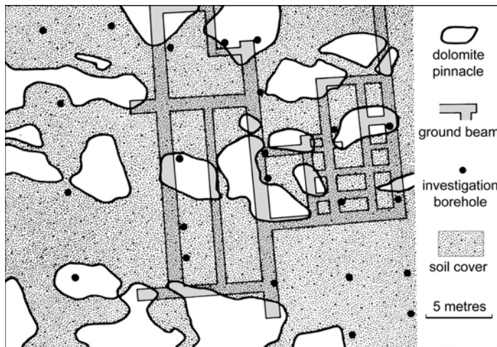
Figure 12.11. Plan view of ground beams designed and extended to reach stable dolomite pinnacles to support a building at Zeerust in South Africa; soils reached more than 20 m deep between the pinnacles. After Brink (1979).
