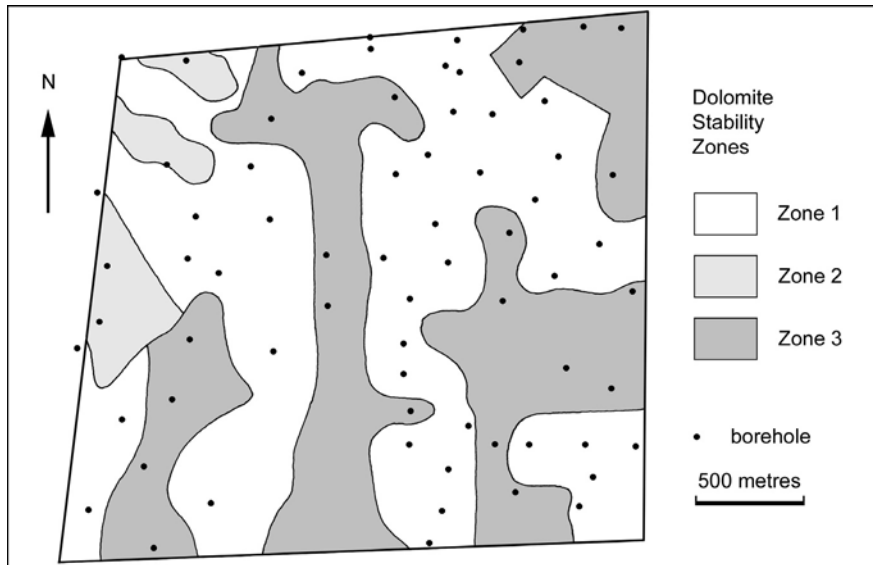
Figure 13.15.3. Division of the Simunye site into three zones with respect to stability and potential sinkhole hazards over the karst dolomite.
