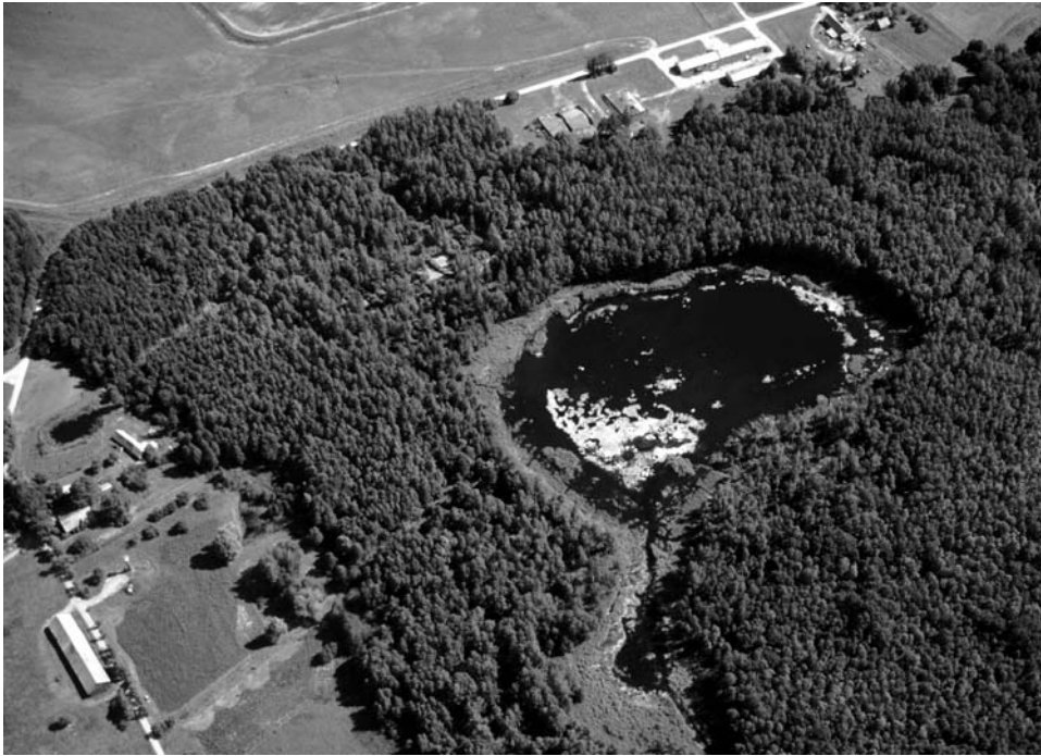
Figure 13.13.1. A large, old, flooded sinkhole in woods surrounded by farmland near Birzai on the soil-covered gypsum karst.
