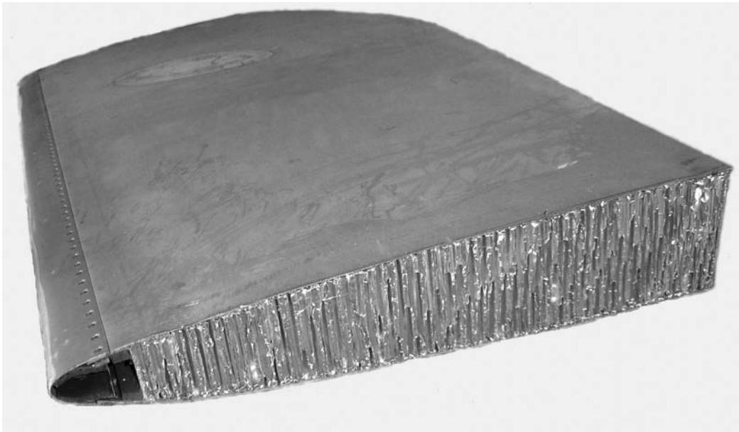
Figure 1.9 A cross-section of a honeycomb structure that plays an important role in the construction of aircraft control surfaces.
