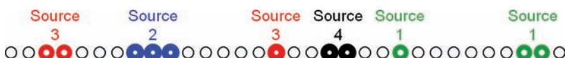
Figure 3.6 Illustration of the properties of a primary sound symbol excitation vector S (only a few of the L components of S are shown). Excited symbols have thicker circles. Each of the four sound sources present (at the moment illustrated) in the auditory scene being monitored is causing a relatively small subset of feature symbols to be excited. Note that the symbols excited by sources 1 and 3 are not contiguous. That is typical. Keep in mind that the number of symbols, L (which is equal to the number of feature vectors) is typically tens of thousands; of which only a small fraction are meaningfully excited. This is because each sound source only excites a relatively small number of sound features at each moment and typical audio scenes contain only a relatively small number of sound sources (typically fewer than 20 monaurally distinguishable sources).
