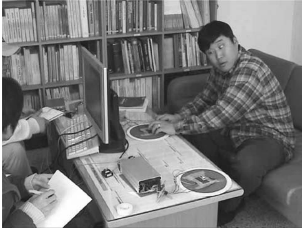
Figure 10.8 Evaluation of the EAP-based braille display device for the visually impaired. (Courtesy of Hyoukryeol Choi, Sungkyunkwan University, Suwon, Kyunggi-do, Korea.)
