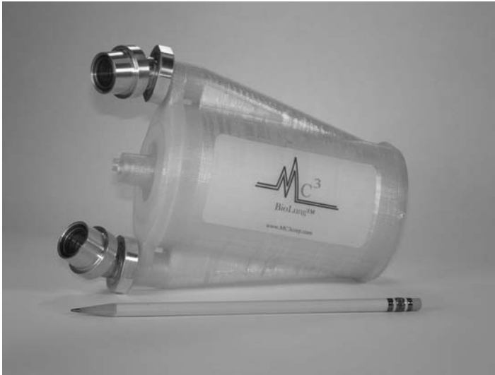
Figure 18.2 The small BioLung artificial implantable lung. (Courtesy of MC3 Corp, Ann Arbor, MI.)
