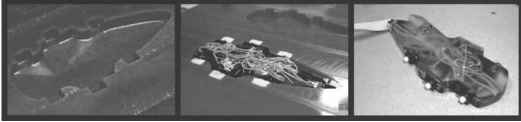
Figure 6.14 Stages in shape deposition manufacture of a small robot at Stanford's Rapid Prototyping and Biomimetic Robotics Labs.
