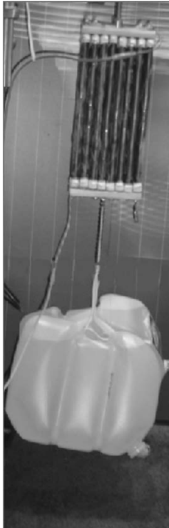
Figure 10.16 One of the groups of EAP actuators made by EMPA lifting two 5-gallon water containers.
