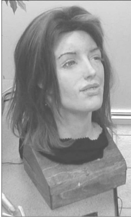
Figure 6.17 (See color insert following page 302) Author's latest robot EVA. Because SPEM silicone requires little force to move, this robot's 36 DOF run for hours on four AA batteries.
