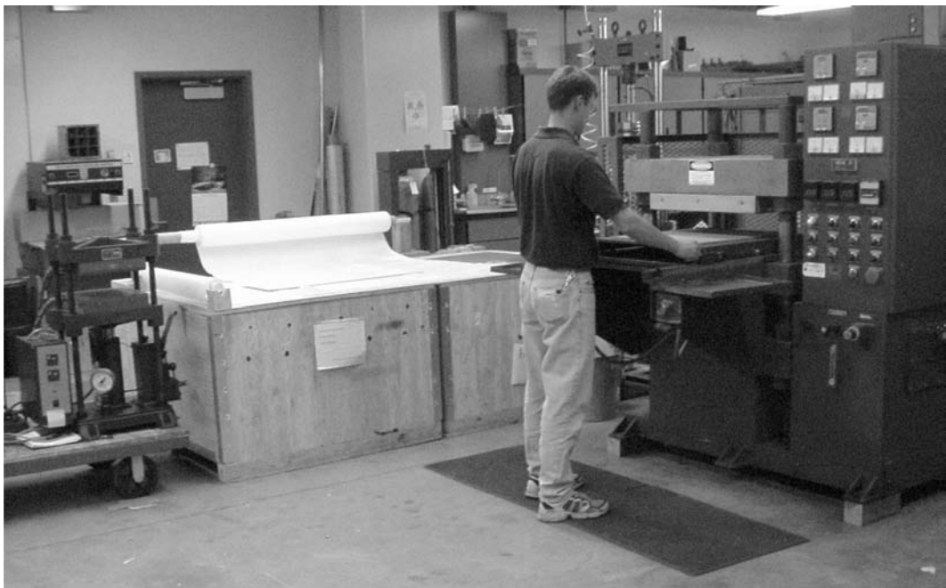
Figure 12.3 (Top) Schematic of two-dimensional thin wire array. One hundred micrometer wires are periodically embedded between composite laminates with layup jig to yield a processed fiberglass/epoxy laminate with array visible inside. (Bottom) Laminating hot presses for processing composite panels.
