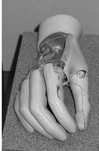
Figure 1.13 A mechanical hand for use as a prosthetic. (Photographed by the author at the Smithsonian Museum in Washington, DC.)
