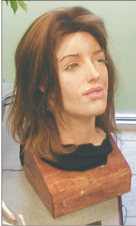
Figure 6.17 Author's latest robot EVA. Because SPEM silicone requires little force to move, this robot's 36 DOF run for hours on four AA batteries.
