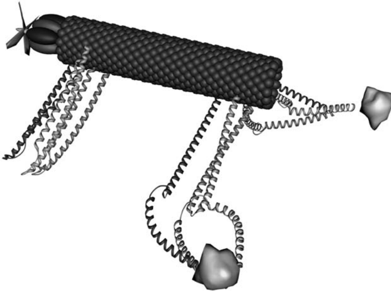
Figure 7.5 The biological elements will be used to fabricate robotic systems. A vision of a nano-organism: carbon nanotubes (CNT) form the main body; peptide limbs can be used for locomotion and object manipulation, a biomolecular motor located at the head can propel the device in various environments.
