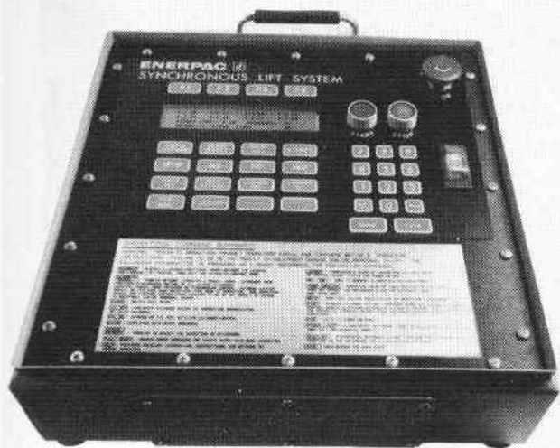
Figure 1-27. PLC unit of synchronous lift system. (Courtesy of Enerpac, Applied Power Inc., Butler, Wisconsin.)
