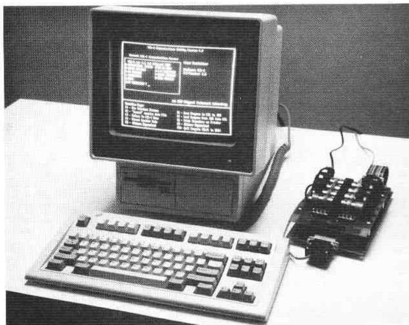
Figure 1-29. PLC system with electronic/pneumatic interface valves. (Courtesy of Clippard Instrument Laboratory, Inc., Cincinnati, Ohio.)
