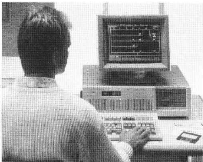
Figure 13-33. Off-line programming of PLC using a microcomputer. (Courtesy of Festo Corp., Hauppauge, N.Y.)
