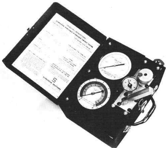
Figure 14-30. Portable hydraulic circuit tester. (Courtesy of Schroeder Brothers Corp., McKees Rocks, Pennsylvania.)
