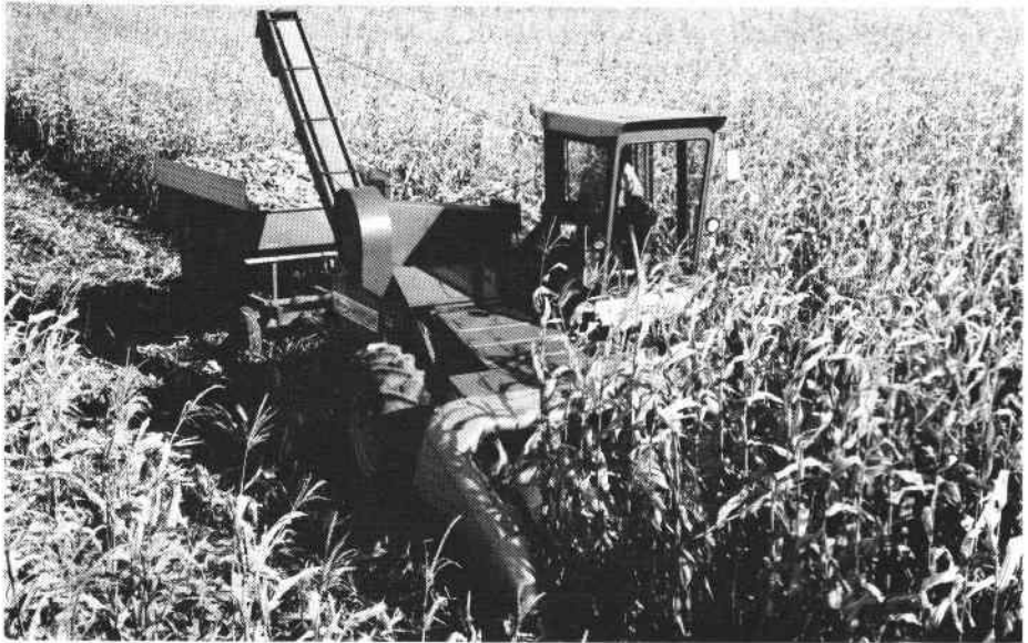
Figure 1-10. Hydraulically driven elevator conveyor for use in harvesting of corn. (Courtesy of Eaton Corp., Fluid Power Division, Eden Prairie, Minnesota.)
