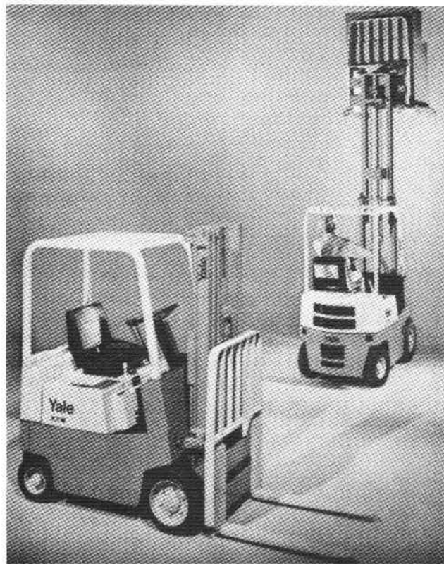
Figure 7-13. High-lift fork truck. (Courtesy of Eaton Corp., Industrial Truck Division, Philadelphia, Pennsylvania.)
