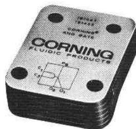
Figure 12-23. AND/NAND gate with its symbol and truth table. (Courtesy of Corning Glass Works, Corning, New York.)
