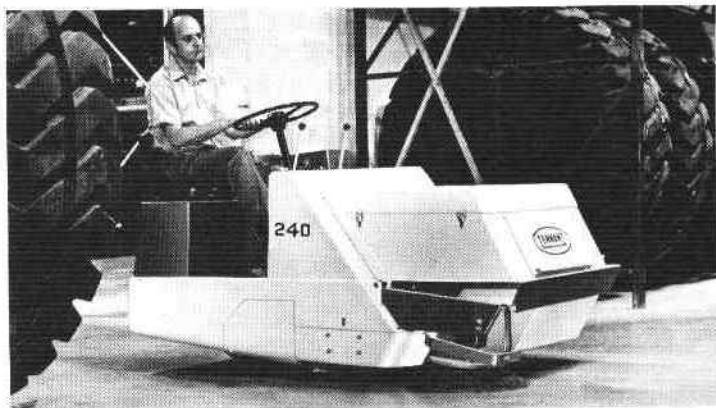
Figure 1-11. Hydraulic power brush drive. (Courtesy of Eaton Corp., Fluid Power Division, Eden Prairie, Minnesota.)
