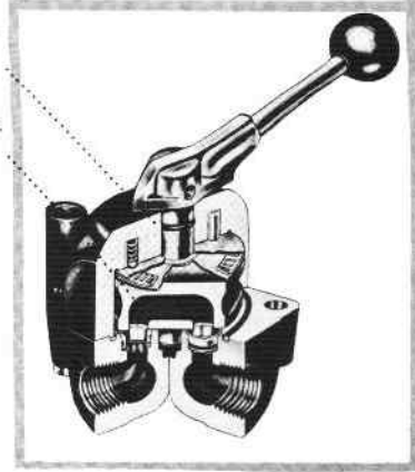
Figure 8-24. Operating features of the shear-flow rotary valve. (Courtesy of DeLaval Turbine, Inc., Barksdale Controls Division, Los Angeles, California.)
