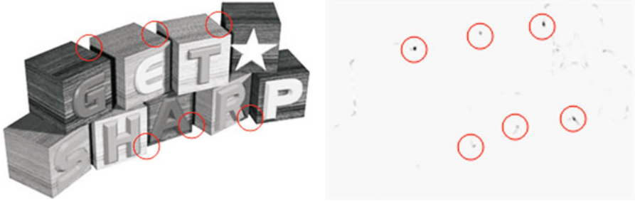
Fig. 7.7. T-junction detection. Left: Image with T-junctions (at the red circles). Right: detection of points with a rapid change of isophote curvature in the gradient direction. This is an example of geometric reasoning for the design of specific features, given their geometric behavior
