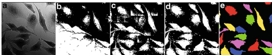
Fig. 1.26. Dynamic thresholding in microscopy [8]. The microscopy of a cell culture (a) was segmented using a global threshold (b), locally adaptive (c) and pixel-adaptive (d). According to morphological post-processing for noise reduction and a connected components analysis, the final segmentation is shown in (e)
