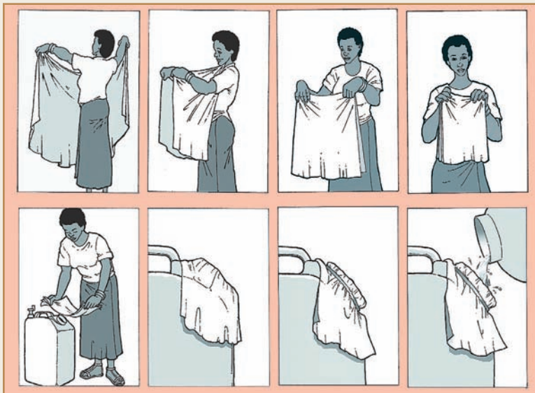
Figure 9.3 Recent studies have shown that filtering water through cloth is an effective way to get rid of harmful microorganisms. This diagram illustrates the proper way to fold the cloth and place it over the mouth of a water jug so that the water will be filtered effectively.
