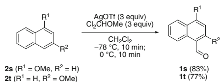
Scheme 4.5 Formylation of methoxynaphthalenes
