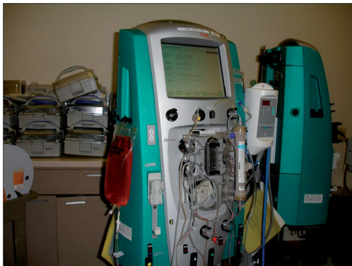
Fig. 34.8 Photograph of a new model dialysis machine that can deliver either intermittent or continuous renal replacement therapy.
