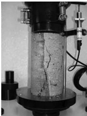
Photo 4.9 Compression test on a cored inter-element sample that shows different colors of self-hardening slurry. (Courtesy of TREVICOS Corp.)
