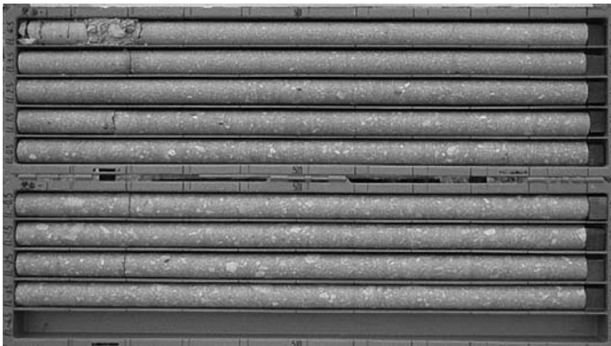
Photo 3.12 TRD core sample from Okinawa, Japan. (Courtesy of Tenox Corporation, Japan.)
