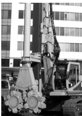
Photo 3.15 Kelly (round) guided CSM unit for depths up to 65 feet.
