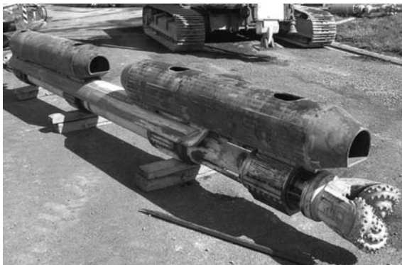
Photo 4.23 The guide connected to the drill-string, Arapuni Dam, New Zealand. (M. Siepi, personal communication, 2011.)
