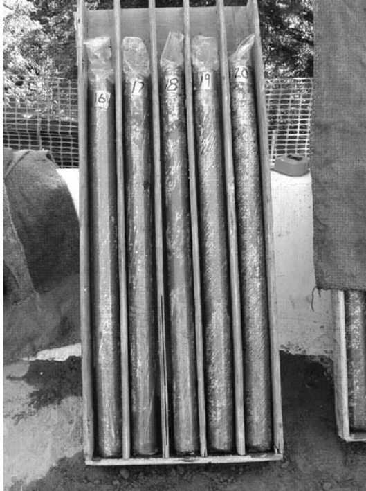
Photo 3.6 Core samples from Sacramento Levee, California. (After Yang, D. S., 5th International Conference on Landslides, Slope Stability & the Safety of Infrastructures, CI-Premier, Kuala Lumpur, Malaysia, 2008.)
