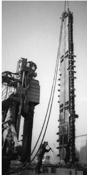
Photo 3.2 TRD “cutting post,” showing the cutting chain to the right, and the carrier machine to the left. (TRD promotional information.)
