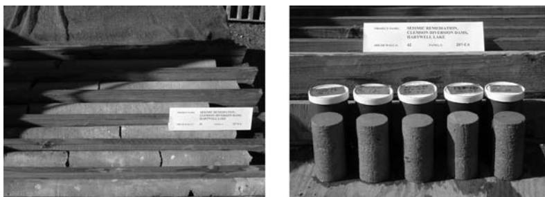
Photo 3.8 Core samples and test specimens from Clemson Dam, South Carolina.
