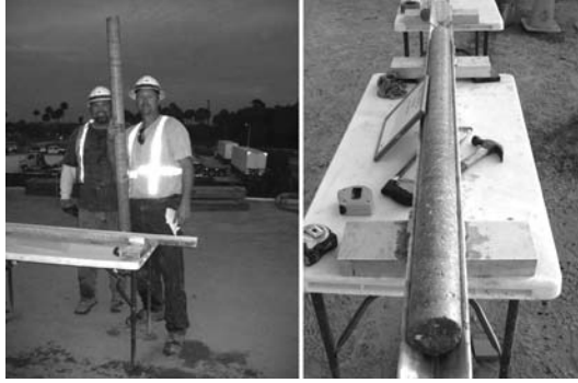
Photo 3.18 Core recovery and samples obtained during CSM demonstration section coring, Herbert Hoover Dike, Florida.
