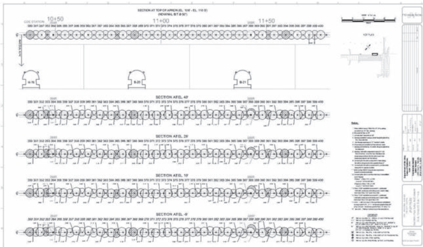
Figure 4.19 As-built drawing of the secant pile cutoff wall at different elevations, W. F. George Dam, Alabama. (Ressi di Cervia, A., "Construction of the Deep Cutoff at the Walter F. George Dam," United States Society on Dams, 25th Annual Conference , Salt Lake City, UT, 2005. With permission.)
