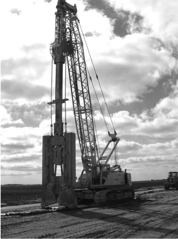
Photo 4.5 Semi Kelly-mounted, hydraulically activated clamshell. (Courtesy of TREVIICOS Corp.)
