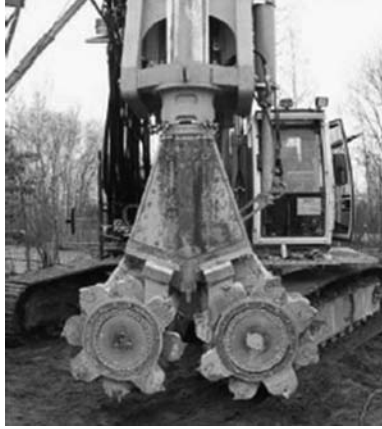
Photo 3.3 The CSM cutter head suspended from a Kelly bar. (Courtesy of Bauer Maschinen.)
