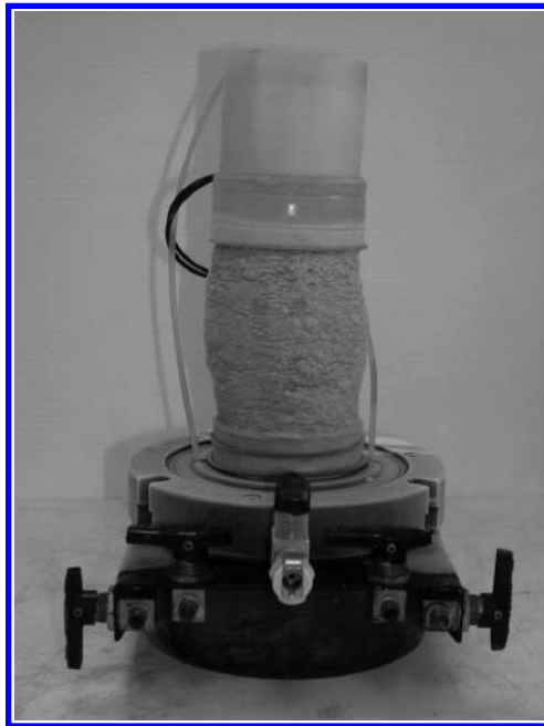
Figure B.13 Triaxial specimen after compression test and freezing.
