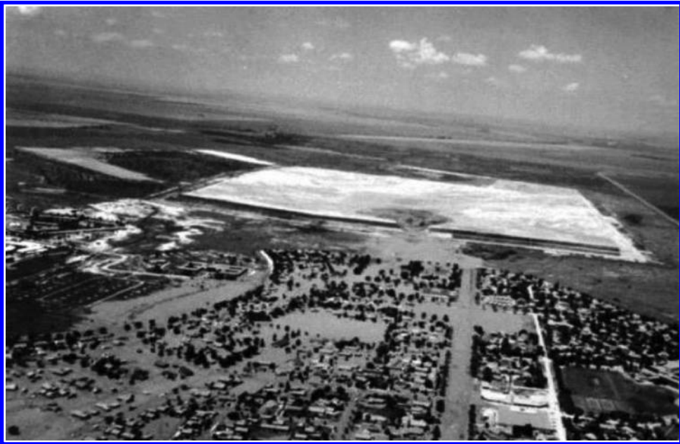
Figure 1.16 Aerial view of the Merriespruit tailings dam failure showing the path of the mudflow that occurred. (From Fourie, A.B. et al., Can. Geotech. J. , 38(4), 707, 2001. With permission from the NRC, Ottawa, Ontario, Canada.)
