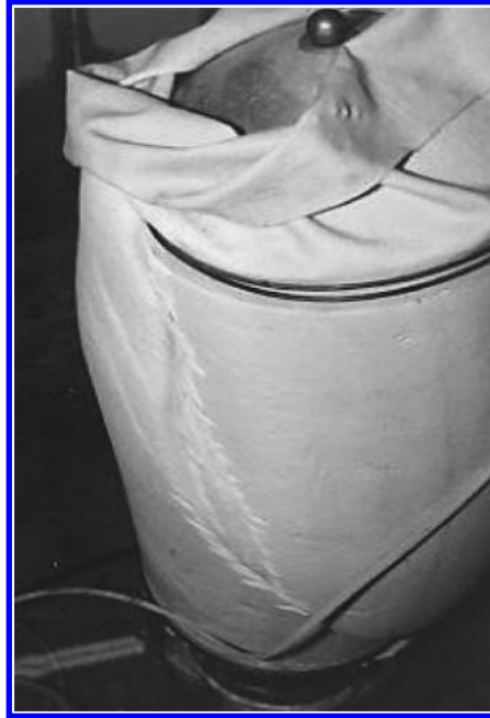
Figure 2.21 Multiple shear bands evident through membrane in large (300 mm diameter) sample after drained shearing.
