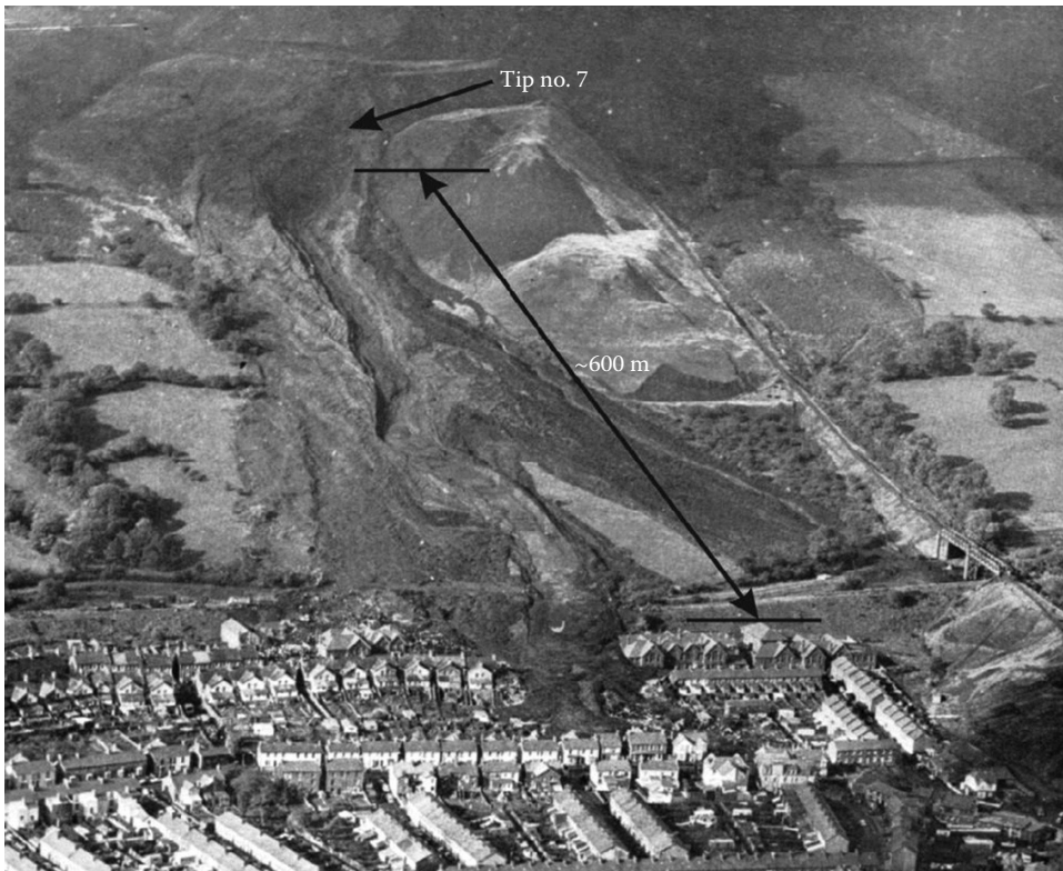
Figure 1.15 Aberfan flowslide shortly after the failure. (Reproduced from Welsh Office, A selection of technical reports submitted to the Aberfan Tribunal, Her Majesty's Stationary Office, London, U.K. With the permission of Controller of HMSO and the Queen's Printer for Scotland; Flowslide distance added by authors.)
