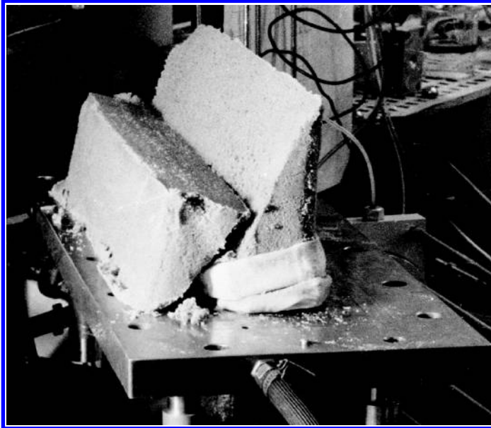
Figure 2.43 Dense sand after failure in Imperial College plane strain apparatus, tested by Cornforth, 1964. (From Cornforth, D.H.: Landslides in Practice: Investigation, Analysis and Remedial/Preventative Options in Soils . 2005. Copyright Wiley-VCH Verlag GmbH & Co. KGaA. Reproduced with permission.)
