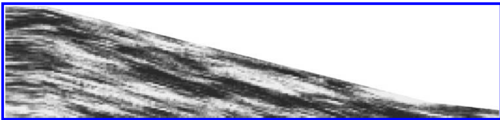
Figure 5.14 Distribution of random \psi field mapped onto Nerlerk berm geometry, computed by Onisiphorou 2000. (Courtesy Dr. M. Hicks, University of Manchester, Manchester, England.)
