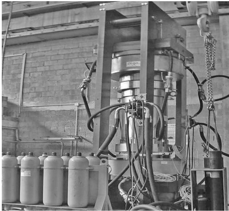
Figure 13.5 Test assembly with an STU in place during the test phase for the Paksey Bridge
