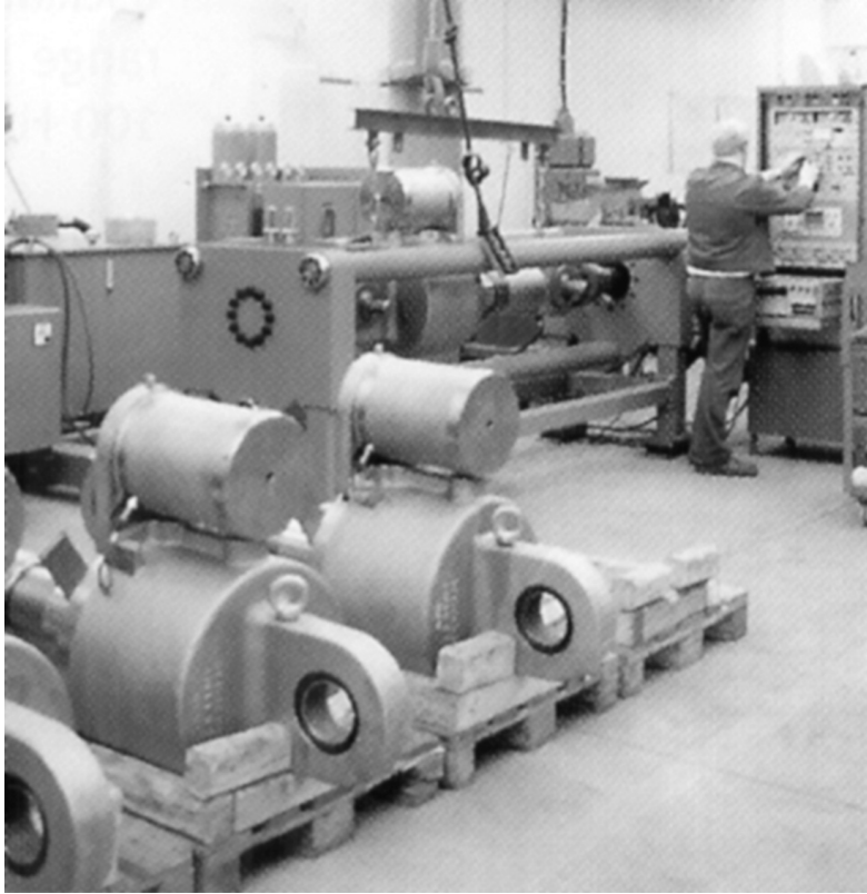
Figure 9.8 Pre-service testing of snubbers in a manufacturer's laboratory
