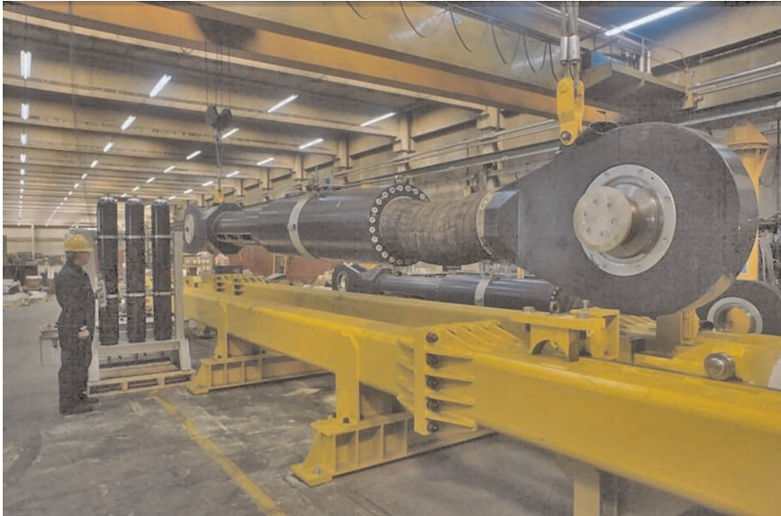
Figure 7.3 One of the 10 m long STUs used on the Storebaelt Suspension Bridge. Reproduced courtesy of FIP Industriale SpA
