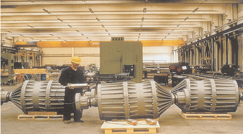
Figure 7.8 The STUs for use on the Second Severn Bridge
