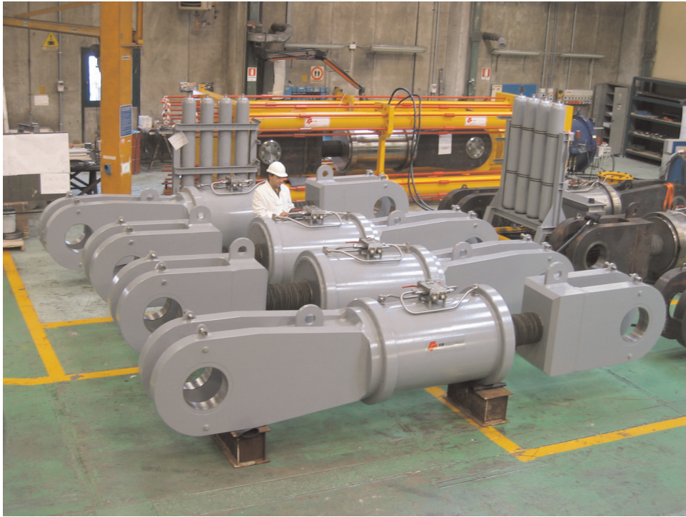
Figure 7.17 The STUs used on Stonecutters Bridge. Reproduced courtesy of FIP Industriale SpA
