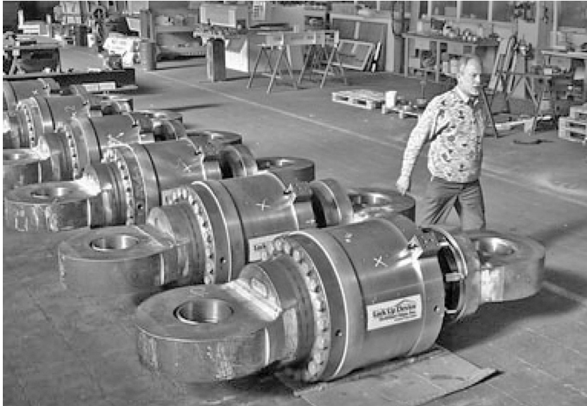
Figure 5.6 The 16 000 kN nominal rated capacity STUs for the Carquinez Bridge ( Use of Lock-Up Devices for Structural Strengthening of the Carquinez Straits Bridge by Warren M. Brown ). © D.S. TechStar, Inc.
