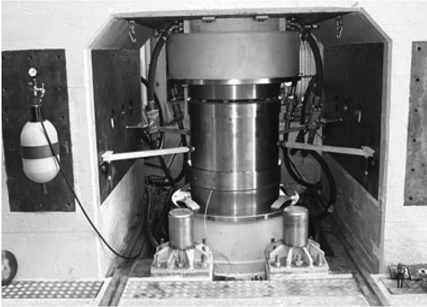
Figure 13.8 One of the TechStar/Alga STUs to be used on the Carquinez Bridge within the test rig for shock load testing
