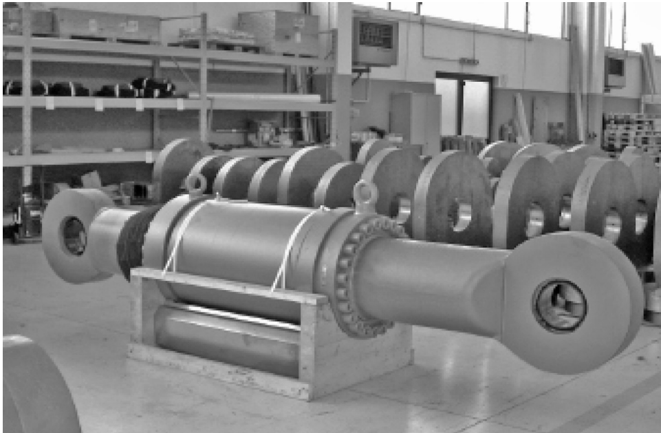
Figure 4.5 A 11 500 kN ULS capacity STU with 750 mm stroke for Paksey Bridge (Hongbing et al. , 2004). © D.S. TechStar, Inc.
