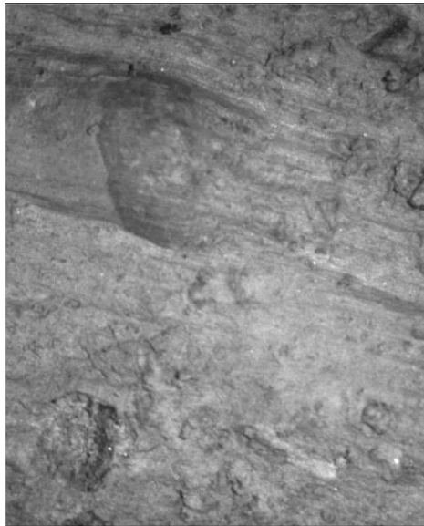
Figure 5.16 Common view from shear surfaces of XT set sheared at moderate and high rate.
