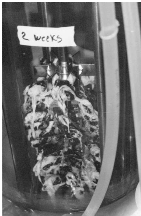
Figure 21.3 Example of Lactobacillus casei biofilm development on PCS tubes mounted on the agitator shaft for repeat batch fermentation. PCS blend employed contained 50% (w/w) polypropylene, 35% (w/w) ground soybean hulls, 5% (w/w) bovine albumin, 5% (w/w) Ardamine Z yeast extract, and 5% (w/w) soybean flour.
