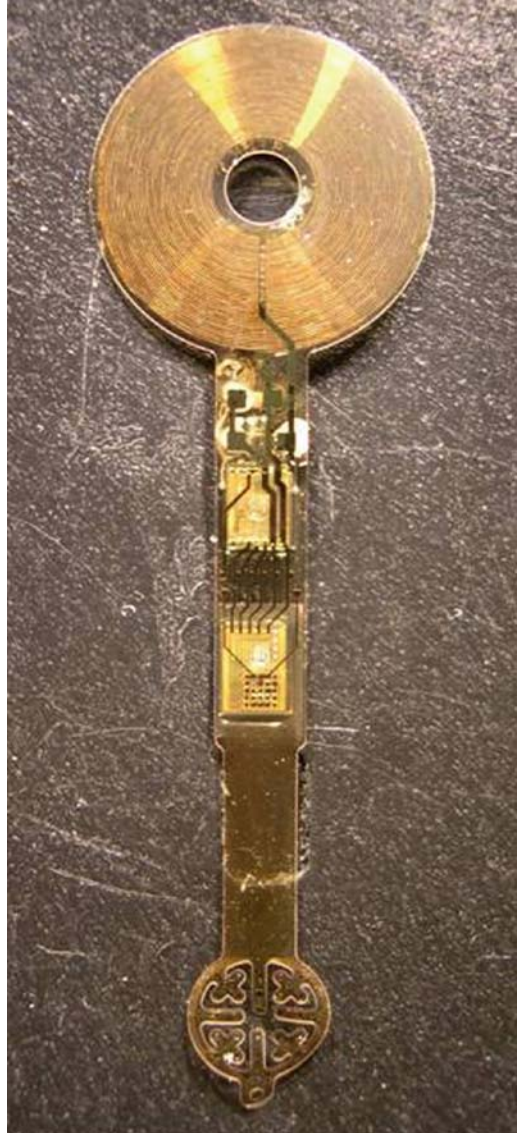
Fig. 12.3 Uncapsulated version of an epiretinal retinal prosthesis with the microfabricated antenna coil for data and energy transfer and the electronic components of the transponder system ( top ) and the microelectrode array with its drivers ( bottom ). Polyimide is used as the basic material. (We acknowledge Professor Peter Walter and the EPI-RET III consortium for providing this figure)
