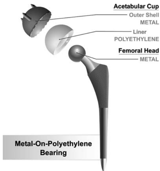
Fig. 13.5 Various components of a THR (figure courtesy of Depuy Orthopedic)
