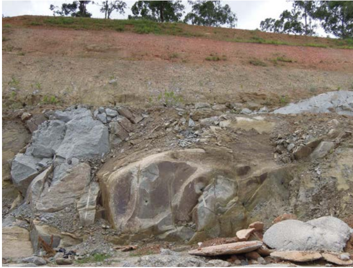
Figure 3.7 Weathering sequence in granite showing irregular surface of fresh granite underlying weathered rock and residual soil (Sao Paulo, Brazil).
