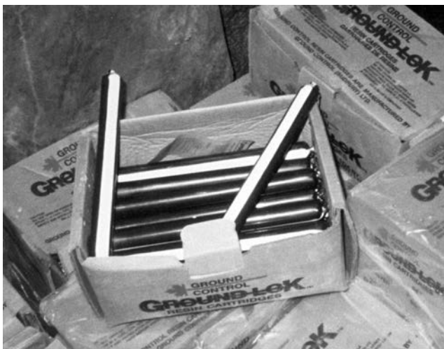
Figure 14.11 Resin cartridges for anchoring rock bolts (Transportation Research Board, 1996).
