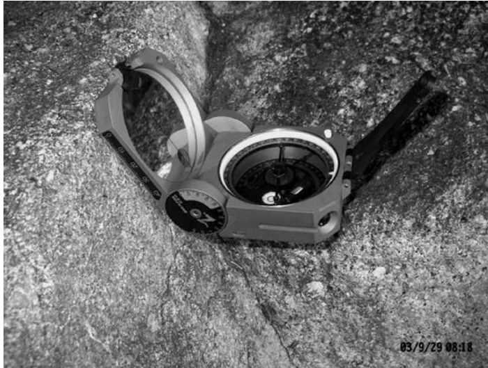
Figure 4.6 Geological compass (Clar type) used to directly measure dip and dip direction of surfaces. Lid is placed on rock surface and body is rotated until it is horizontal, as indicated by the spirit level; the needle is released to indicate dip direction, and the dip is read off scale on the hinge (The Brunton Co., Riverton, Wyoming).
