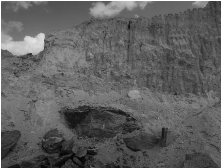
Figure 3.1 Cut in weathered rock showing core stones of slightly weathered rock in matrix of highly weathered rock (Recife, Brazil).
