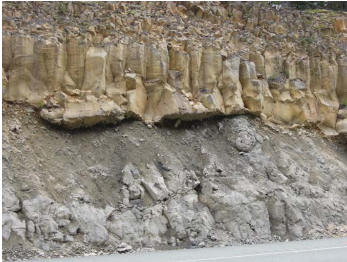
Figure 3.9 Columnar basalt flow overlying weathered soil that has undermined the basalt (Sea to Sky Highway, British Columbia, Canada).
