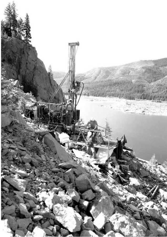
Figure 4.1 Typical diamond drilling equipment drilling vertical hole, with core logging being conducted on site. (Image by Norman Norrish.)
