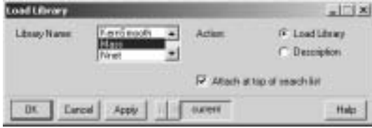
Figure A.1: The dialog box to load the MASS library. Note that the check box is ticked.
