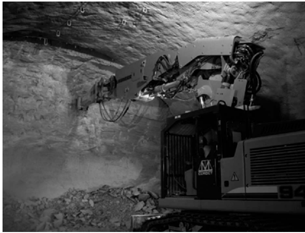
Figure 9 Typical Impact Hammer Mounted on an excavator.
