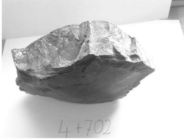
Figure 5 Traces of tectonic stresses on rock samples taken from the zones where the TBM is squeezed.
