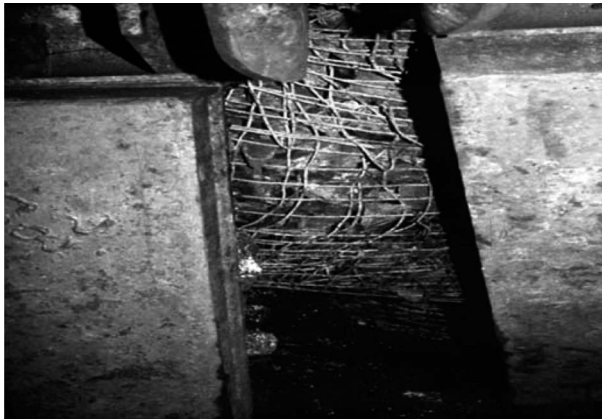
Figure 8 Mesh visible between shield supports.
