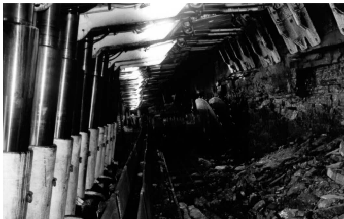
Figure 15 4.8m high SPL face at West Wallsend Colliery (after Hamilton, 1999).
