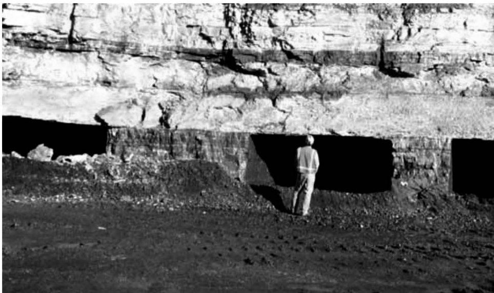
Figure 7 Highwall mining, showing a barrier pillar (left) and a web pillar (right).
