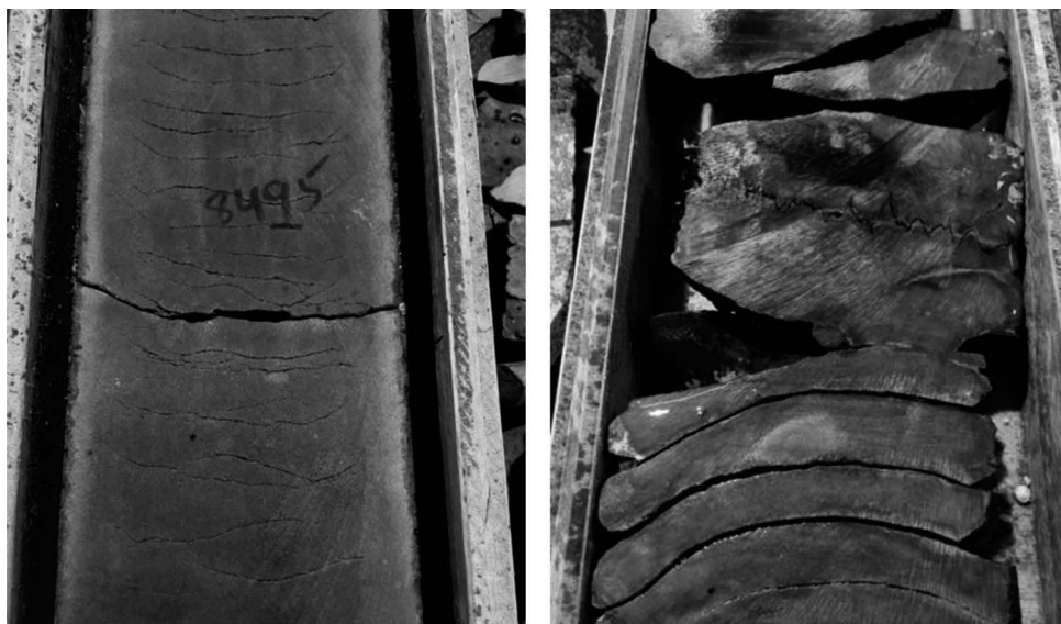
Figure 10 Examples of incipient core disking and well developed disking in a core of lower cretaceous formation, Onshore Abu Dhabi.
