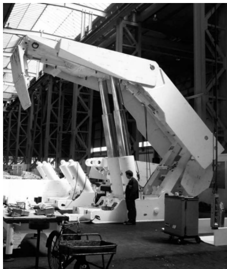
Figure 16 DBT 6m supports for Matla Mine, South Africa (photograph courtesy of DBT).
