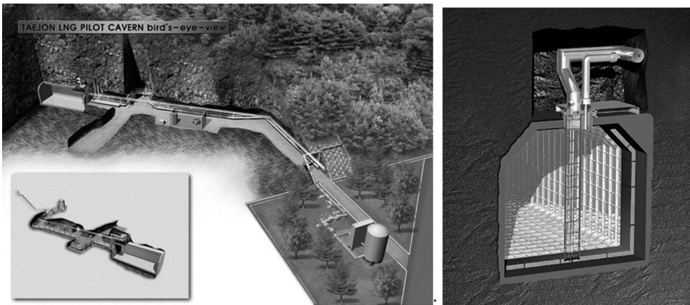
Figure 7 A bird's-eye view and cross section of the pilot cavern (Park et al., 2010).
