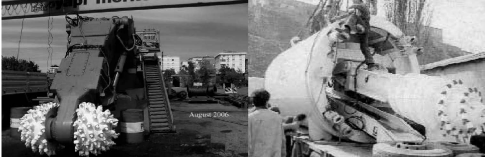
Figure 8 Typical roadheaders used in Metro stations (left transverse type) and utility tunnels (right axial type).
