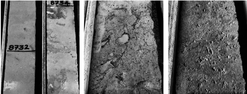
Figure 18 Cores cut from lower cretaceous carbonate reservoirs from onshore Abu Dhabi in the United Arab Emirates, illustrating the heterogeneity within formations.
