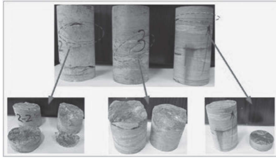
Figure 2 The damage phenomenon in the process of freeze-thaw test.
