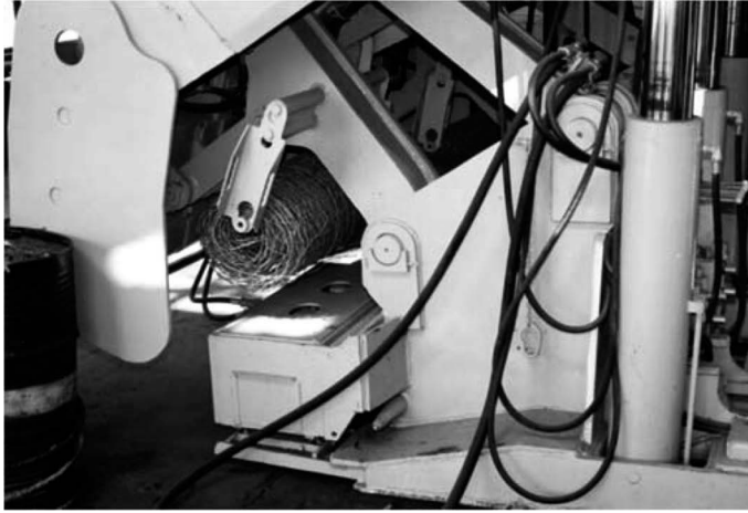
Figure 7 Wire mesh placement behind top slice of MSL face.
