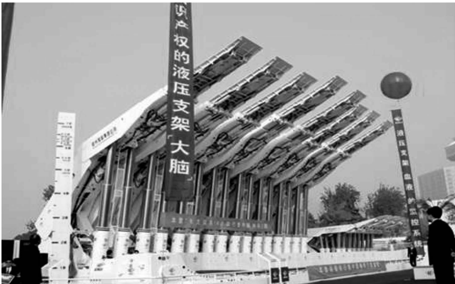
Figure 17 Bulianta Mine 7m high face supports (photograph courtesy of Shenhua).
