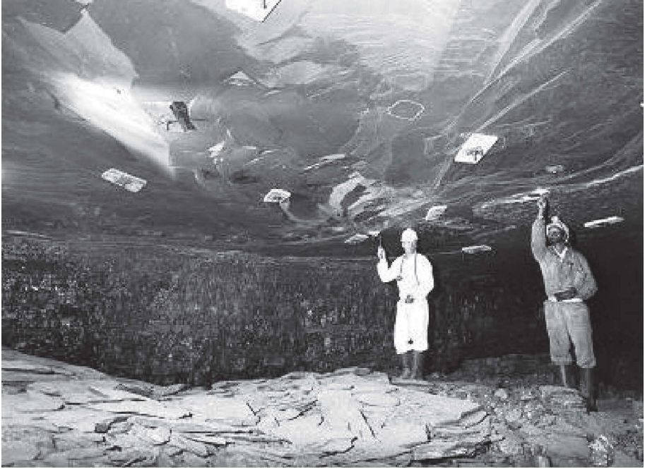
Figure 4 Illustration of violent failure in competent rock at very low stress levels (Stacey et al., 2007).
