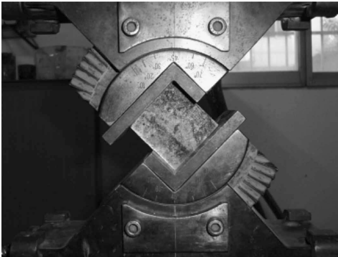
Figure 18 The spherical seats used for shearing which can be rotated at different angles.
