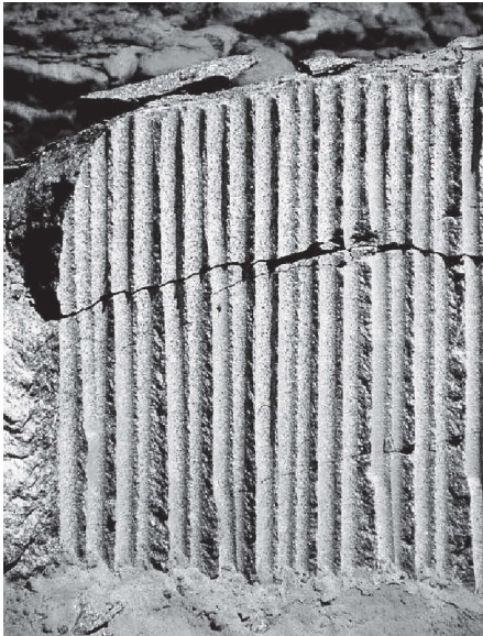
Figure 5 Illustration of violent fracture development in a quarry (Stacey et al., 2007).
