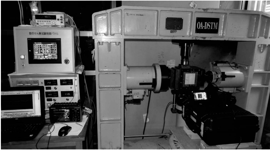
Figure 6 Multi-purpose dynamic shear-testing machine with an ability to perform creep tests on rocks, discontinuities and interfaces at the University of the Ryukyus.
