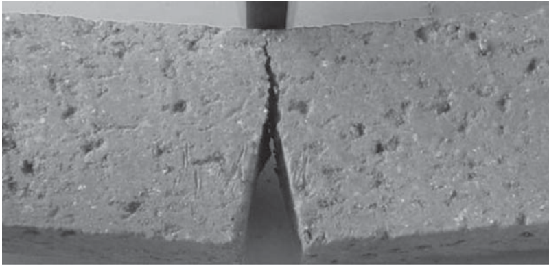
Figure 4.5 Crack shape of single edge cracked beam after rupture
