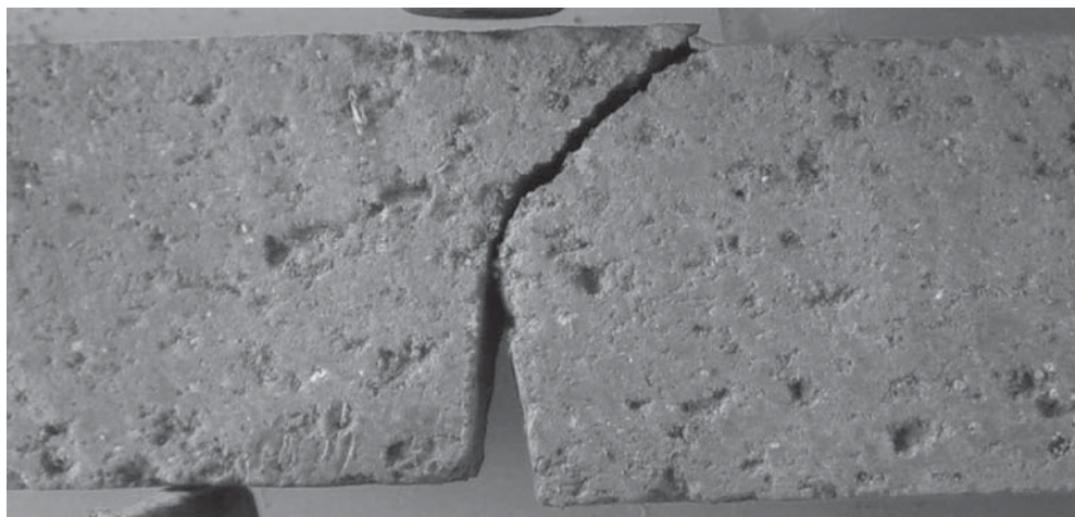
Figure 5.2 Crack shape after fracture failure of the specimen in mode II
