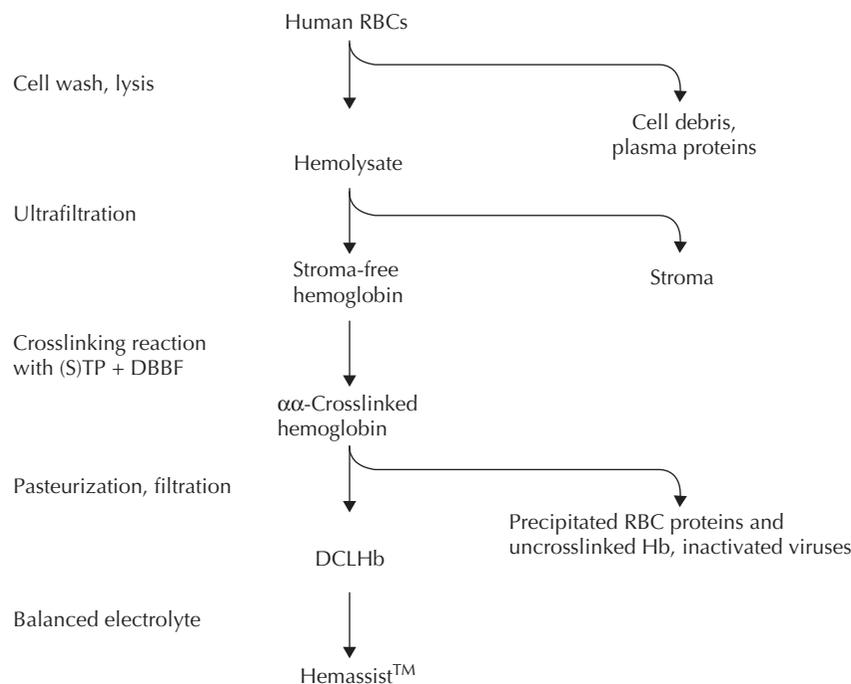
**Figure 34.1** Schematic diagram of the HemAssist™ manufacturing process.
