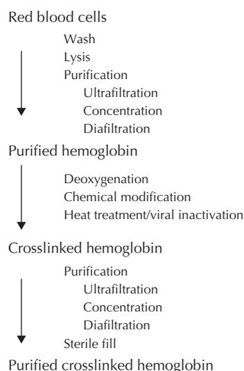
**Figure 33.1** Flow chart for the production of human hemoglobin crosslinked between the  $\alpha$  chains  $\alpha\alpha$ -Hb. From Hess *et al.*, 1993.
