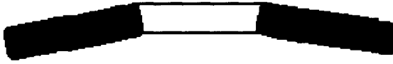
Figure 2-12. The Belleville washer's shape allows it to apply high loads to anchor bolts
