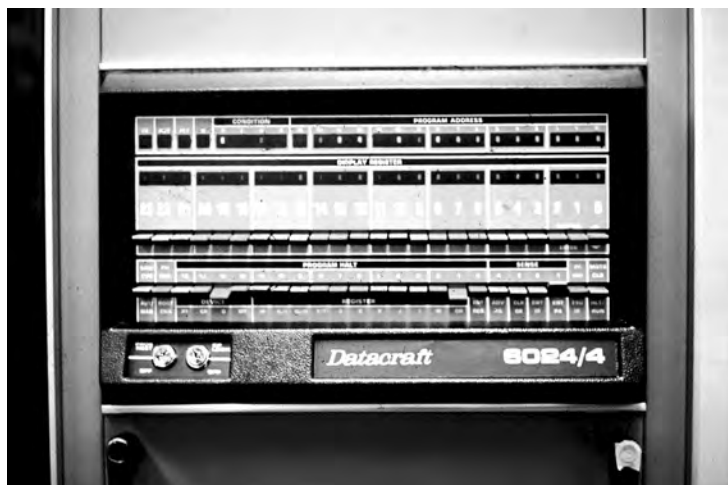
Fig. 1.2. The minicomputer revolution in computational chemistry began as machines like this Datacraft 6024/4 at the University of California (1973) came into use. This was a 24-bit machine (48 bits per word in extended precision). Note the two rows of switches. These could be used to directly set the bit strings for one word of memory at a time, a low-level feature that at least proved helpful for certain crashes.
