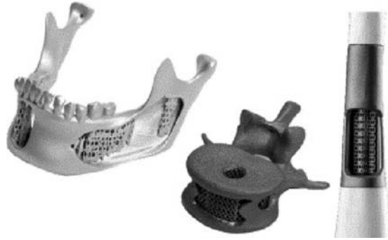
Fig. 6.6 A stainless steel parts of a lower jaw, lumbar vertebra, a middle segment of the tubular femoral bone produced by selective laser melting
