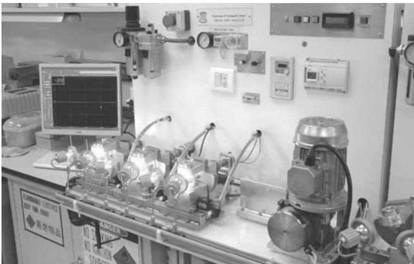
Fig. 9.12 Joint motion simulator for wear testing
