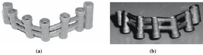
Fig. 8.33 The 4-implant dental bar: (a) wax pattern; (b) metal bar cast from Ni-Cr alloy (Liu et al., 2006)
