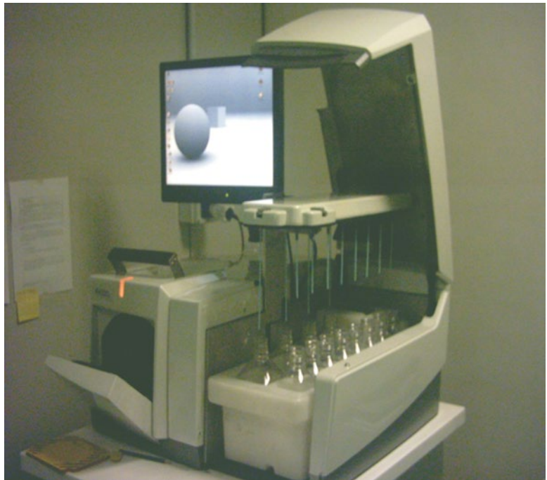
Fig. 9 The FLX-Titanium Roche/454 sequencer. The fluidic part at the right side and the signal detection device in the left side
