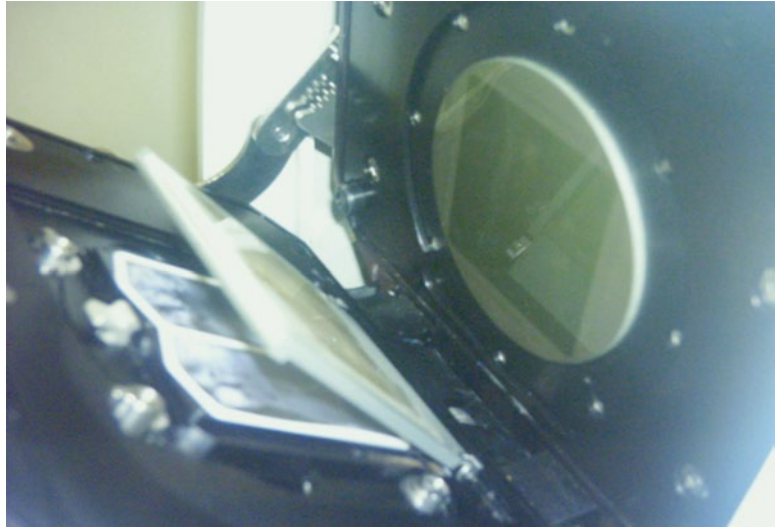
Fig. 10 The signal detection device in the left part of the sequencer. The PTP loaded inside the cartridge, located in front of the CCD camera
