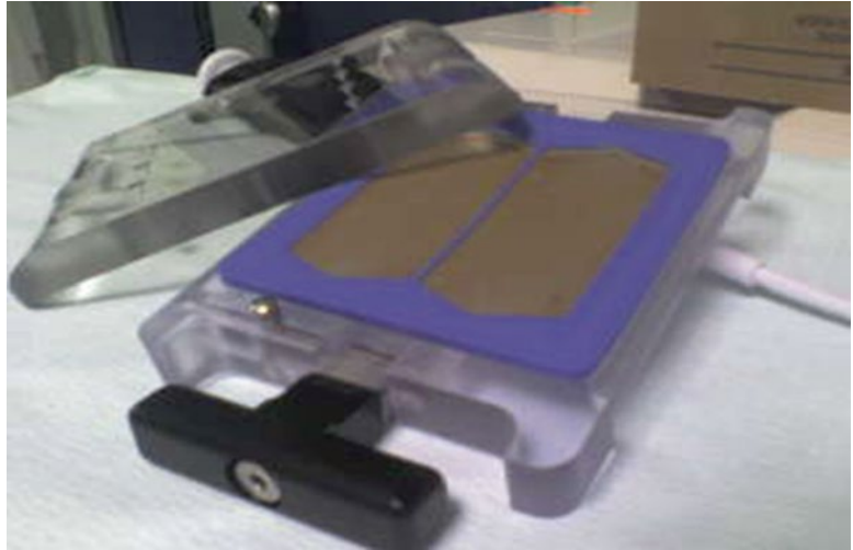
Fig. 8 The Beads Deposition Device (BDD) used to load the sample beads and the PTP divided into two regions
