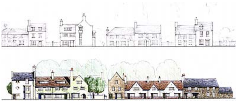
Top: Initial architectural elevations reflect the use of local construction materials and vernacular detailing
