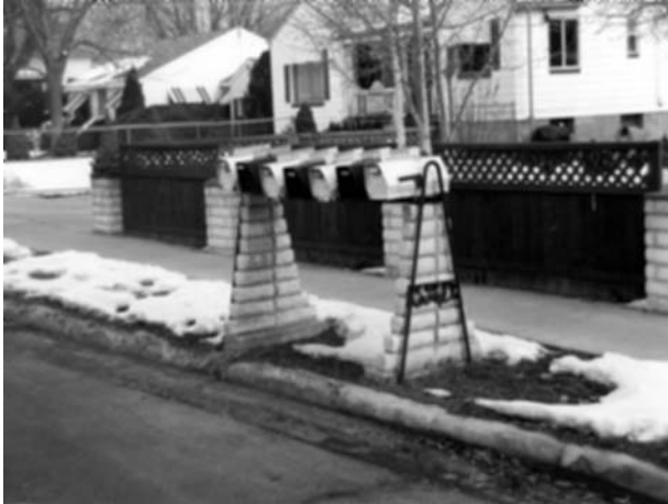
FIGURE 11.3 Examples of hazardous multiple mailbox installations
