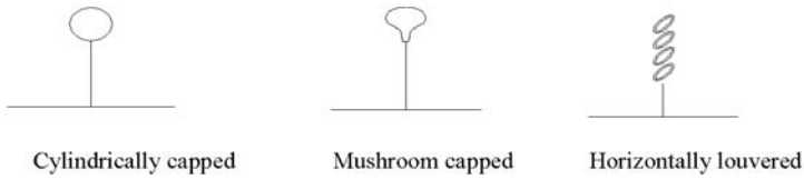
Figure 6.10 Schematics of barriers with absorptive treatment, cross-sectional view. Adopted from Ekici (2004).
