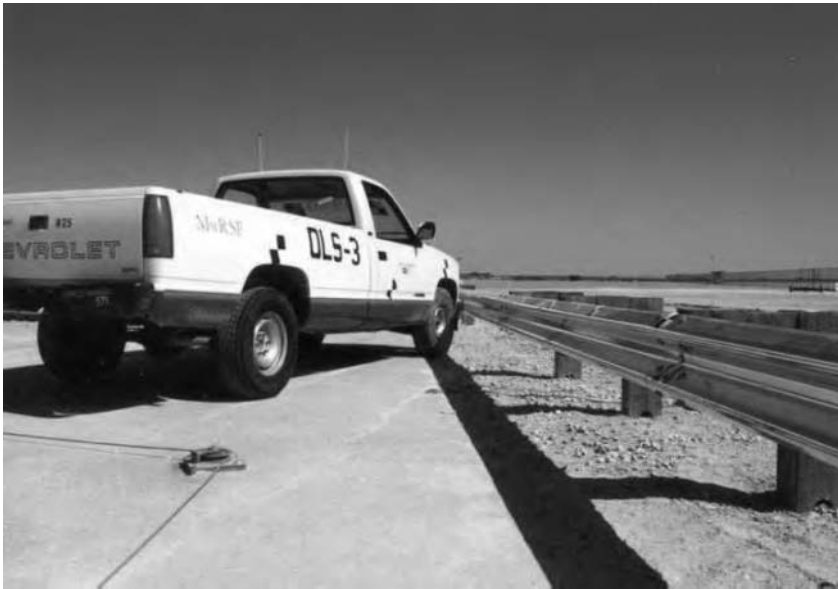
Figure 5-25. Long-Span, Nested W-Beam Guardrail
