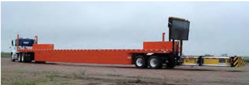
Figure 9-31. Mobile Barrier Trailer
