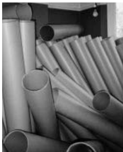
Figure 2.21 Cardboard tubes for insertion in boreholes to isolate piles from swelling of soil
