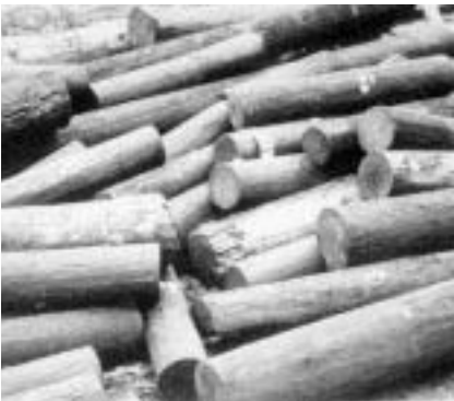
Figure 4.29 Redundant transmission poles removed for investigation of durability
