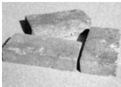
Figure 6.7 Fired clay pavers of two different thicknesses, 50 and 63 mm, made in the West Midlands in the 1920s
