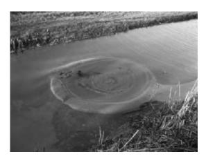
**Figure 3.6.** Sand boil during high water period of 2011 (Hurwenen, The Netherlands)
