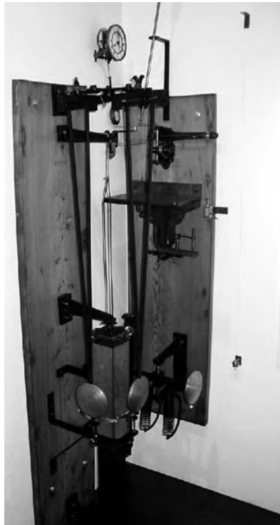
Fig. 28.3 The Cecchi electrical seismograph with sliding smoked paper (Cecchi 1875), after restoration
