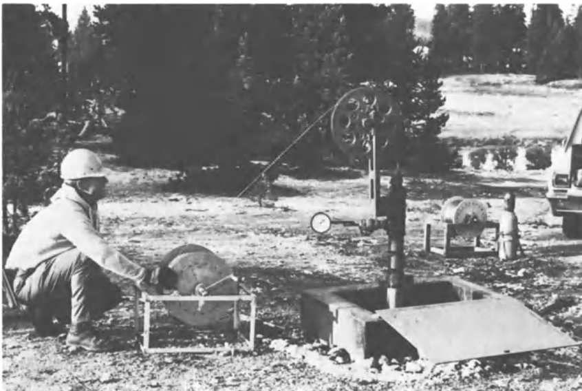
Figure 2.8. Sampling from a drill hole in Yellowstone Park. Stainless steel tubing is lowered to the desired depth from the reel in the operator's hands.
