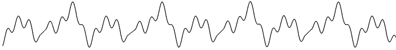
Fig. 3.10 The effect of a window on the signal for FFT in Fig. 3.9
