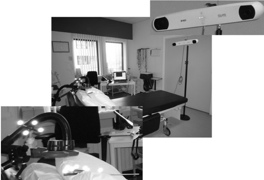
Fig. 11.6 Example of a set-up for neuronavigated rTMS. The subject will be positioned on the bed. The TMS coil with the attached cooling system and the pointer (enlarged on the bottom left ) at the head-end of the bed are both fitted with reflecting spheres that can be recognized by the camera (enlarged on the top right ) at the foot-end of the bed. Note that since the photo was taken with a flash, the spheres actually reflect in the photo
