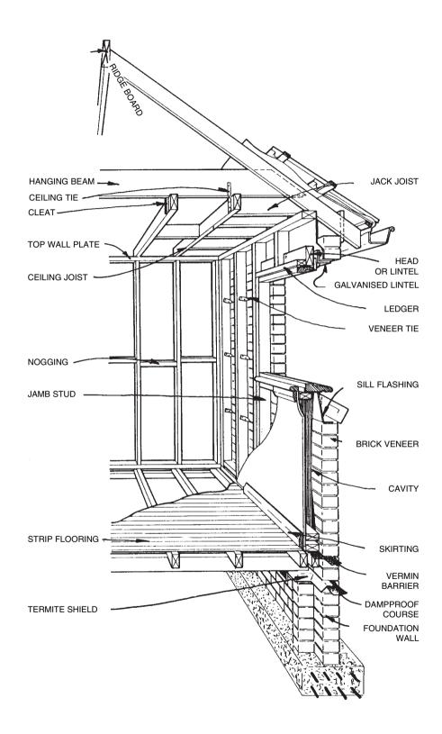
Figure 3 Brick veneer construction
