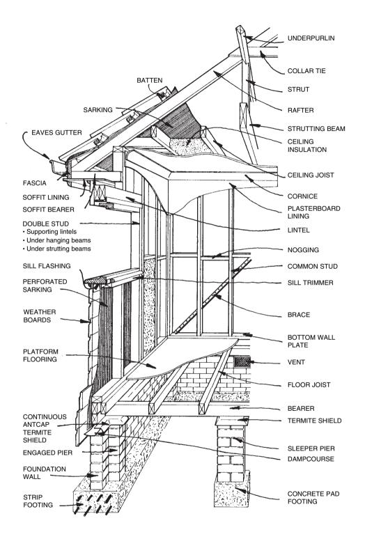
Figure 2 Timber framed construction
