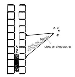
Figure 16.1 Cone device for removing honey bee activity from a cavity wall
