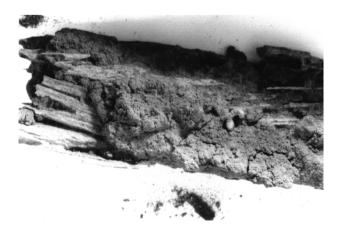
Figure 21.1 Eucalypt hardwood damage caused by lucanid decay borer
