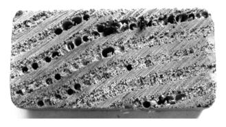
Figure 21.4 Solitary bee — damage to the softer growth rings of a Douglas fir roofing member
