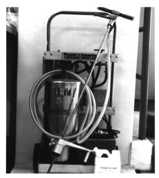
Figure 9.4 B+G Trouble-Shooter Portable Foaming Unit
