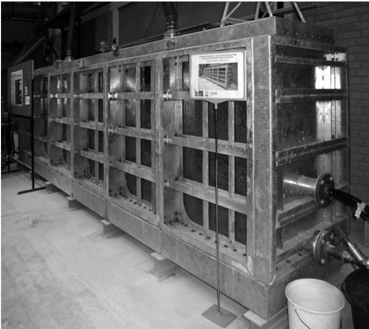
Figure 15.8 An installation for testing of fiber-optic cable for the purpose of seepage detection in the hydraulic laboratory of Innsbruck University (September, 2010).
