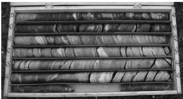
Figure 2.8 The drilled core at one borehole below Knezhevo dam (Macedonia), depth 39 to 45 m.
