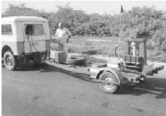
Figure 14.10 FWD testing in progress: National Highway 1.
