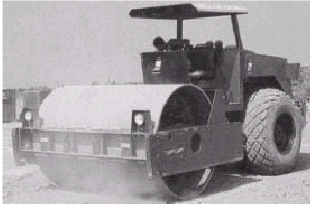
Figure 13.7 A vibratory roller under work.
