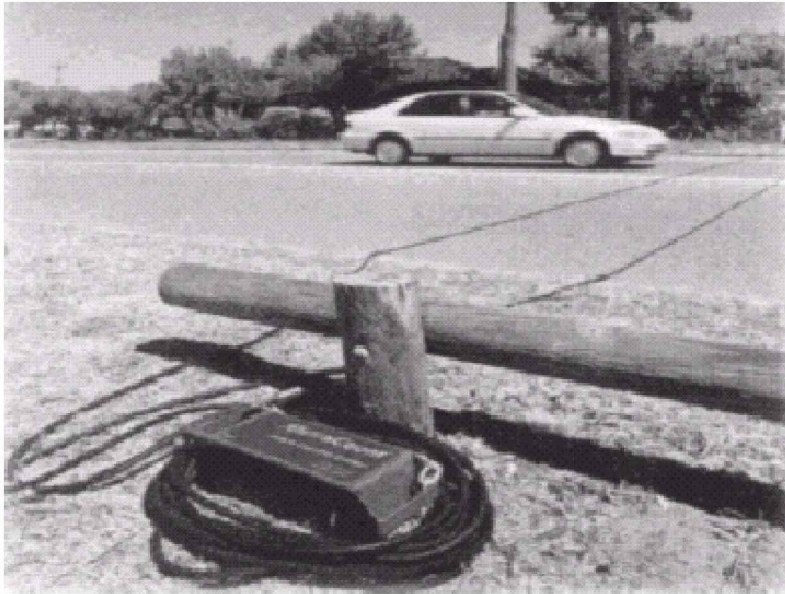
Figure 4.5 A typical tubular presence type detector.
