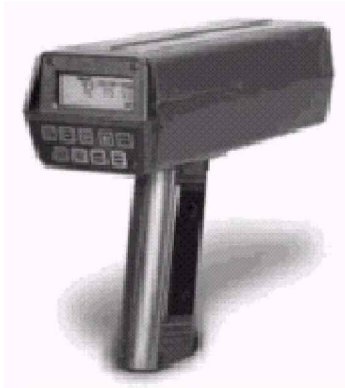
Figure 4.4 A typical speed gun which measures the spot speed of vehicles.
