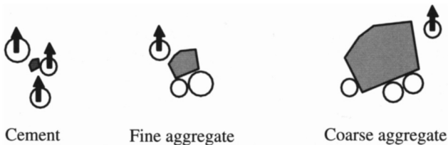
Figure 2.27 Mechanism of air entrapment during consolidation.
