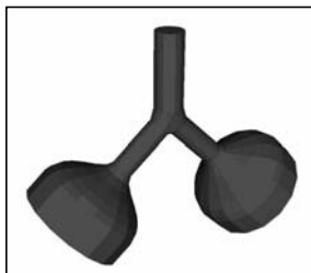
Figure 6: Two generations geometry used in this section. The piston-like structures at exits simulate lung pumping.
