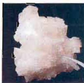
▲ Figure 2.14 A sodium chloride crystal. The sodium ions ( \text{Na}^+ ) and chloride ions ( \text{Cl}^- ) are held together by ionic bonds. The formula \text{NaCl} tells us that the ratio of \text{Na}^+ to \text{Cl}^- is 1:1.
