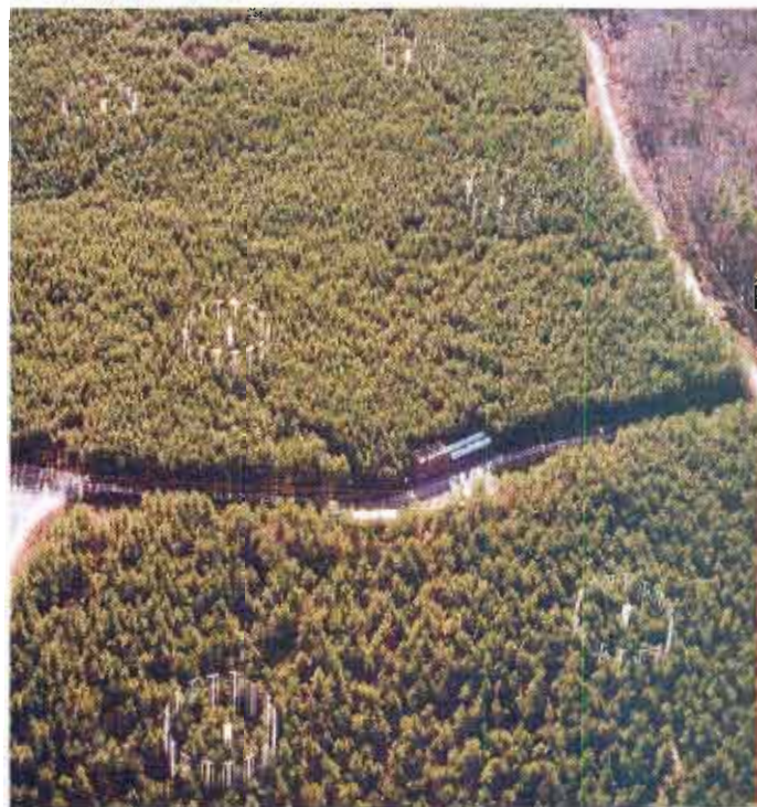
▲ Figure 54.25 Large-scale experiment on the effects of elevated CO_2 . Rings of towers in the Duke University Experimental Forest emit enough carbon dioxide to raise and maintain CO_2 levels 200 ppm above present-day concentrations.
