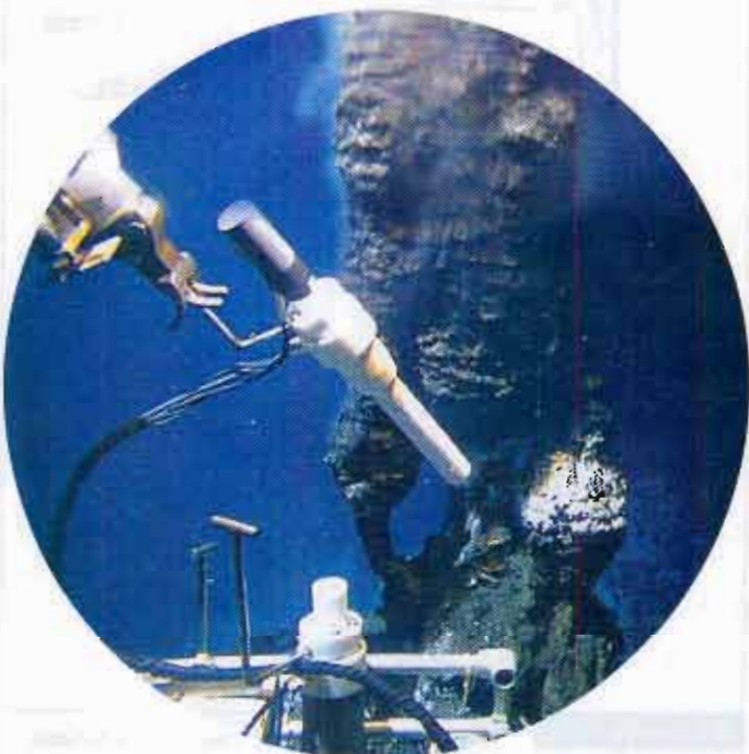
▲ Figure 26.3 A window to early life? An instrument mounted to a robotic arm on the research submarine Alvin samples the water around a hydrothermal vent in the Sea of Cortés. More than 1.5 km below the surface, the vent releases hydrogen sulfide and iron sulfide, which react and produce pyrite (fool's gold) and hydrogen gas. Prokaryotes that live near the vent use the hydrogen as an energy source. Such environments are among the most extreme in which life exists today, and some researchers favor the hypothesis that life may have begun in similar regions of early Earth.
