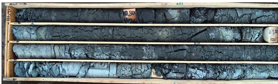
Figure 5.3 Early deterioration of rock core.
