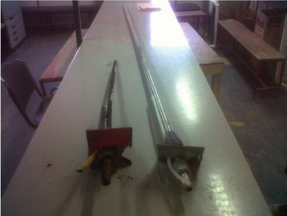
Figure 9.7 Corrosion of rock bolts from direct contact of acidic groundwater.
