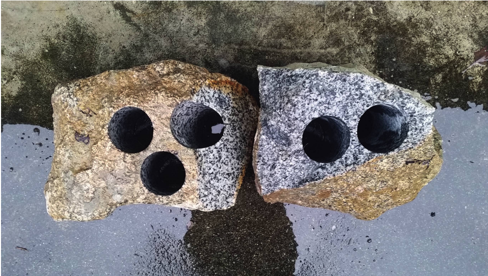
Figure 4.10 Rock block sample for testing of drillcores.
