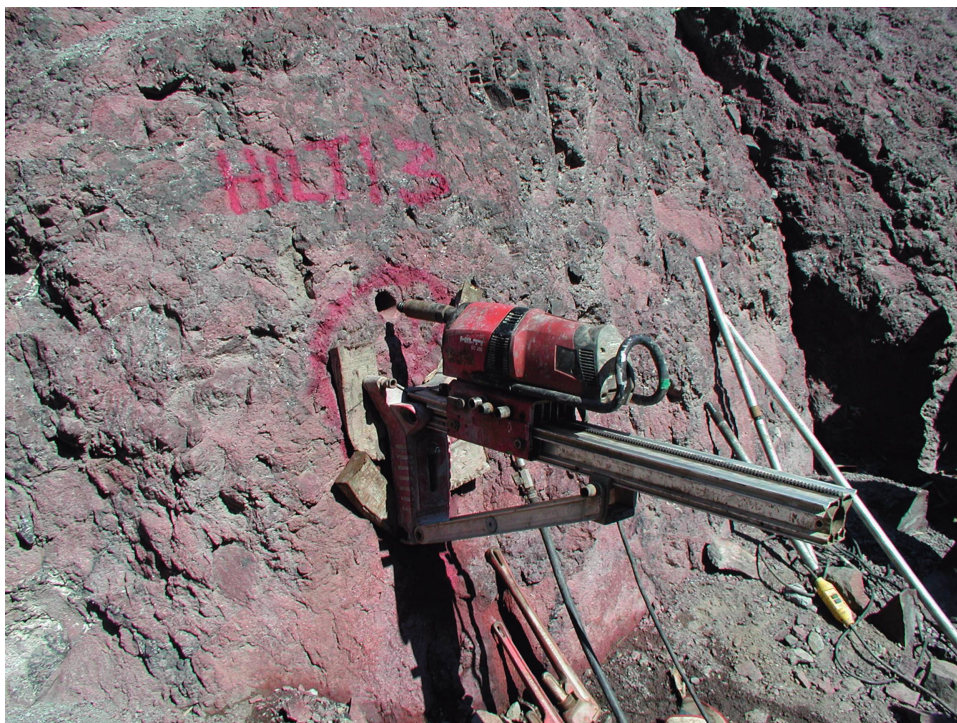
Figure 4.11 Portable drilling rig for short drillholes for samples.
