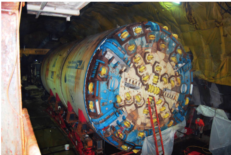
Figure 8.8 Single shield TBM.
