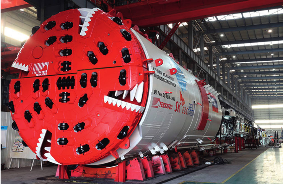
Figure 8.7 Double shield TBM.
