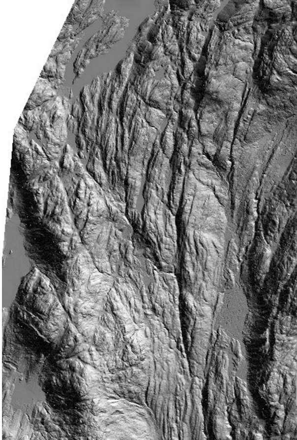
Figure 4.2 LiDAR example for identification of geological faults.
