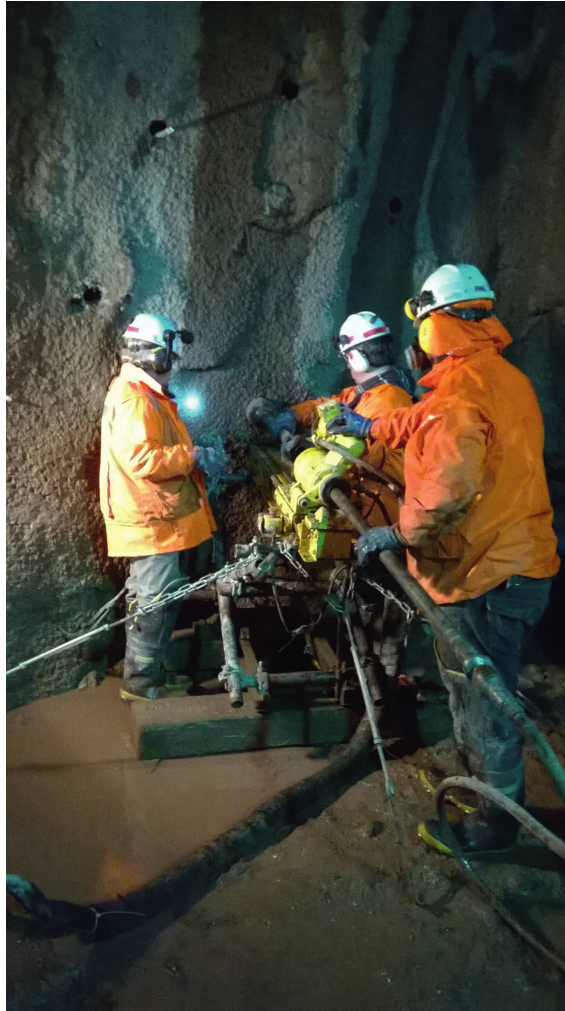
Figure 4.9 Overcoring in situ stress testing.
