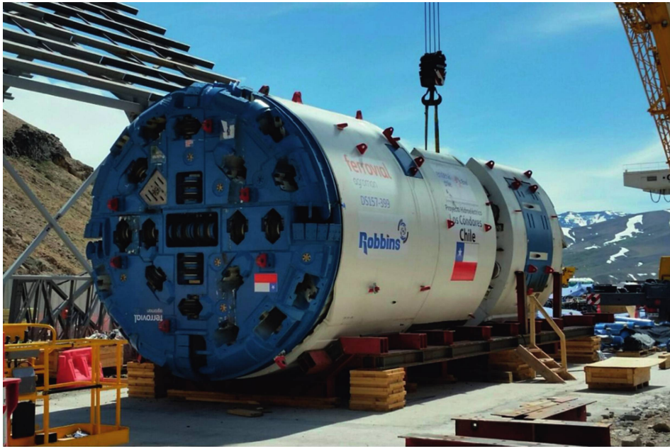
Figure 19.17 Double shield TBM for practical construction and lining of non-durable rock.
