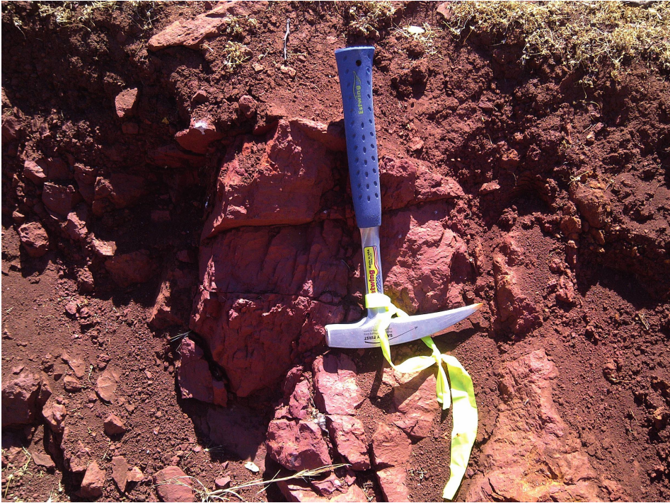
Figure 19.14 Non-durable red tuffs in outcrop.
