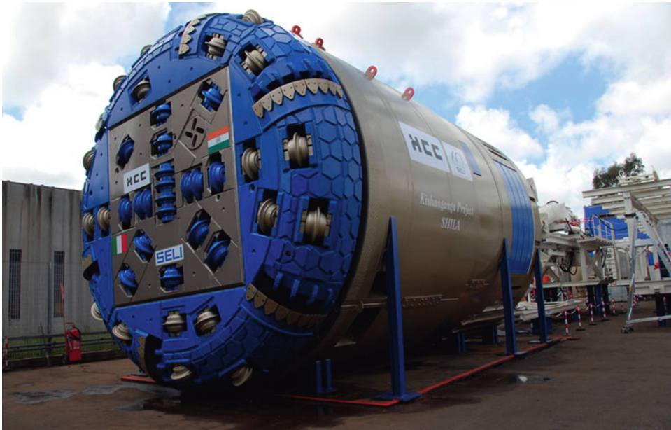
Figure 8.9 Double Shield Universal (DSU) TBM.
