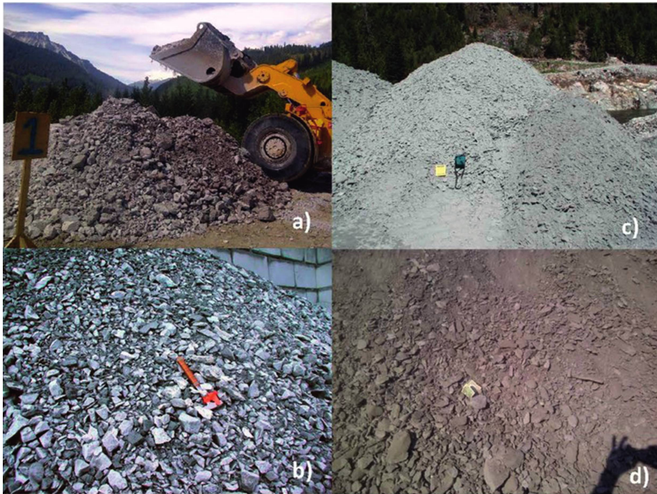
Rock spoil a) drill and blast, b) TBM, c) raisebore, d) roadheader
