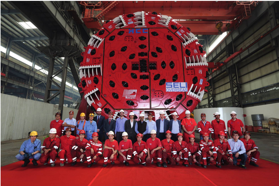
Figure 3.1 Double shield TBM for the 12 km Vishnugad Pipalkoti Hydropower Project.
