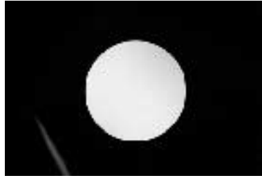
Figure 2.1. A jam-pot cover placed between crossed polaroids may form a bright, clear 'window' by twisting the polarisation direction through 90^\circ . Rotating the cover by 45^\circ in either direction 'closes the window'.
