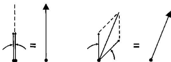
Figure 8.13. If one of the rotating vectors of figure 8.12 is delayed a little, they will meet up at a different point and so the resultant linear vector will be rotated. This shows that circular birefringence (when two circular vectors propagate at different speeds so that one of them is delayed) in sugar solutions rotates the direction of linearly polarised light as seen in the equivalent phenomenon of optical activity described in chapter 5.
