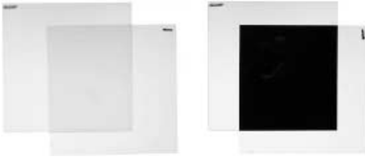
Figure 1.3. One polariser, a sheet of polaroid film, only allows half of the random, unpolarised light to pass but this is then all vibrating in one direction. Such polarised light passes easily through a second polaroid that is aligned with the first (left) but is completely blocked when the two polaroids are crossed (right). This simple but striking demonstration can easily be demonstrated to an audience on an overhead projector.
