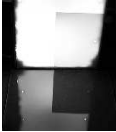
Figure 7.1. Polarisation by reflection in a sheet of glass. A vertical light box (a backlit translucent screen) has a piece of polaroid propped against its lower right, with the polarisation direction vertical. Light from the screen reflects well from a horizontal sheet of clear glass and also passes quite well through the polaroid. But light from the polaroid is not reflected in the glass because it is incident at around Brewster's angle at which only horizontally polarised light can be reflected.
