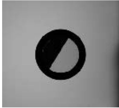
Figure 8.7. A Cotton circular polariscope for detecting whether light is circularly polarised and its handedness, here seen over a circular polaroid background film. Two pieces of circular polaroid, one left-handed and the other right-handed, are simply mounted next to each other. The device must be viewed from the side bearing the linear polaroids, otherwise it acts as a linear polariscope (see figure 1.4). If circular polaroid of only one handedness is available, half of it can be covered with a suitably orientated half-wave film to change its handedness. Another alternative is to mount two pieces of linear polaroid, with their directions at right angles, over a single, properly orientated quarter-wave retarder film.
