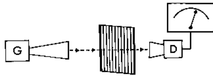
Figure 1.2. Apparatus to demonstrate polarisation with microwaves. A generator produces electromagnetic microwaves (3 cm wavelength radio waves) that vibrate in one direction only. A tuned receiver detects these waves only if they vibrate in one direction as shown by the deflection on a meter dial. With the two devices aligned, the meter is deflected, but detection ceases when either of them is twisted by 90^\circ around their common axis. A grid with spacings less than the wavelength allows the waves to pass in one orientation but blocks them when it is turned onto its side around the axis of the beam.
