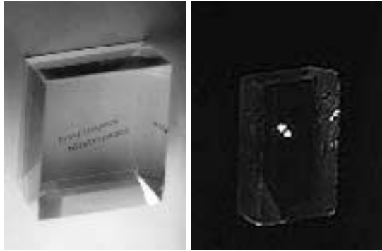
Figure 3.4. Left: a calcite crystal over a single typed word on a sheet of paper, showing a clear double image. This spectacularly large, clear crystal belongs to the Royal Institution, whose help is gratefully acknowledged. Right: a smaller calcite crystal over a small hole in a black card. In both cases, rotating a polariser over or under the crystal would extinguish each image in turn, showing that they are polarised at right angles to each other.
