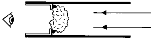
Figure 6.4. A possible sunstone—a ‘natural’ polariscope made from a cordierite crystal. A screw bottle top with a hole cut in it supports the rough crystal within a short cardboard tube. The direction of polarisation in the crystal can be determined with a piece of polaroid and marked on the outside of the tube. The direction of the sun can then be found by pointing the tube at the sky and watching the crystal darken as the tube is rotated. Compare this device with the ‘synthetic’ version shown in colour plate 7.
