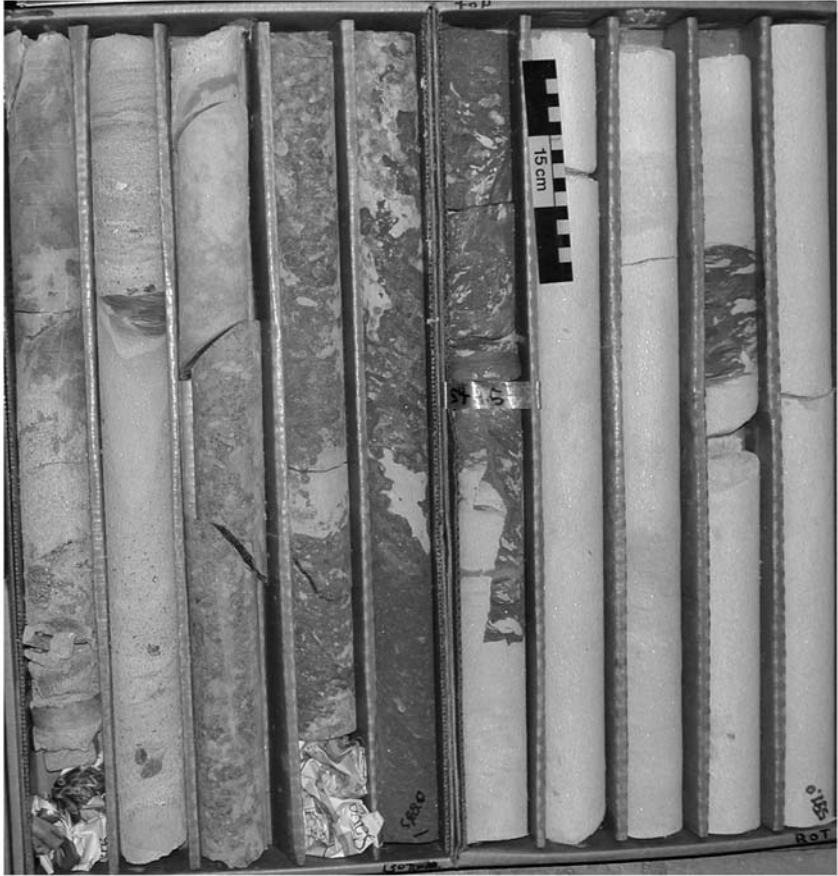
Fig. 5. Core from Schroeder well, at Wetumpka impact crater center, showing most of a ~6-m Tuscaloosa Group target rock block. Interval is -164.1 m to -169.7 m (upper left to lower right). Mottled interval in upper part of center three cores contain Taenidium in bioturbation. Light grey = sand; Dark grey = red clays. 15-cm scale bar.
