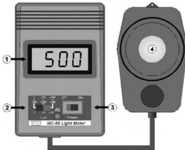
Figure 12.11 Diagram of a typical lightmeter, showing LED display (1), range switch (2), on/off switch (3) and the photocell (4)
