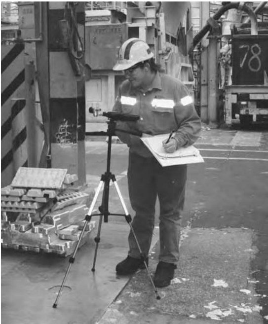
Figure 12.2 Use of a portable WBGT in an indoor industrial setting
