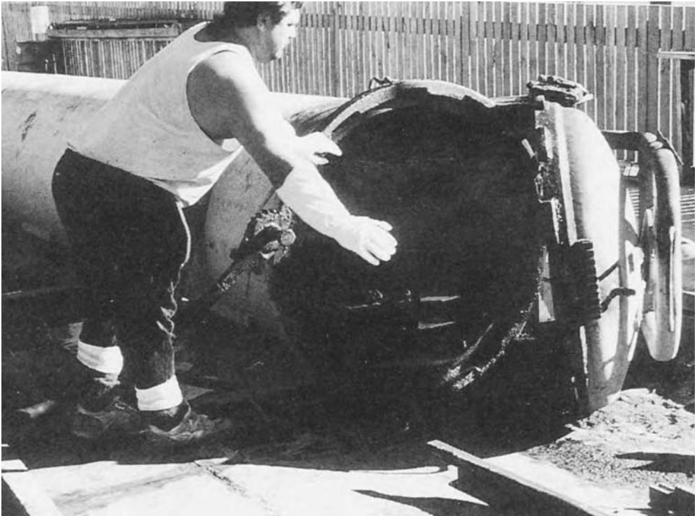
Figure 6.4 Gauntlet hand-arm protection is required when handling arsenic-treated timber
