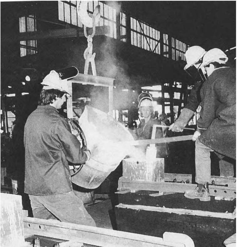
Figure 6.1 Brass founding may result in some exposure to lead fume
