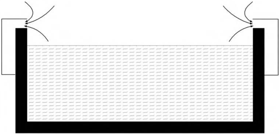
Figure 4.21 Slot hoods along the length of a tank
