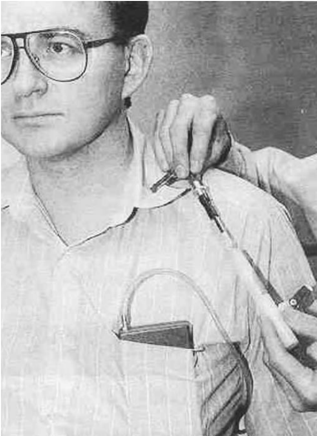
Figure 7.11 Worker being fitted with a sample pump and adsorbent tube
