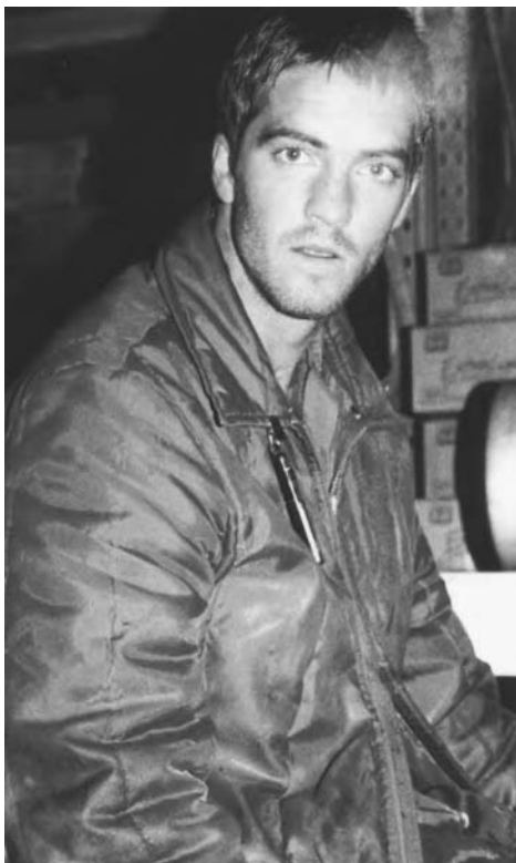
Figure 7.3 Personal direct reading passive monitoring tube on an operator's lapel close to the breathing zone
