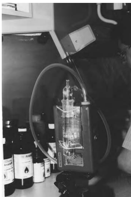
Figure 7.16b Sample pump and liquid impinger (on side) for trapping gases in a laboratory
