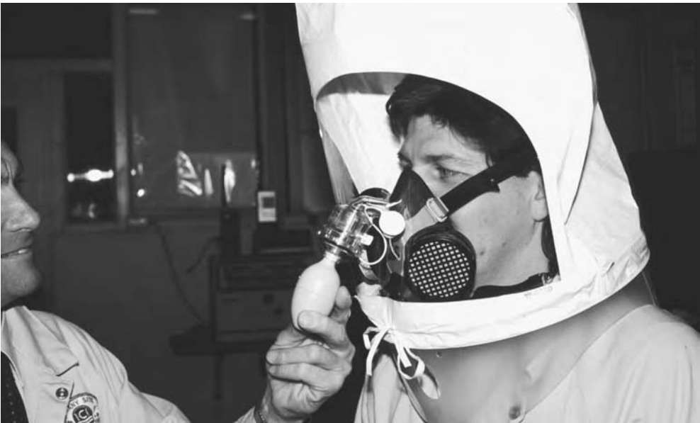
Figure 4.8 Qualitative facial fit testing using a saccharin aerosol
