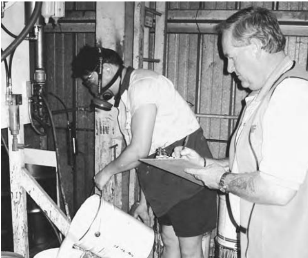
Figure 1.1b Conducting a walkthrough survey in a drum plant; observing the process of preparing automatic spray-painting machines
