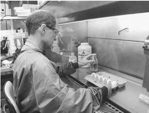
Figure 13.4 Laboratory worker using a Class II Biological Safety Cabinet
