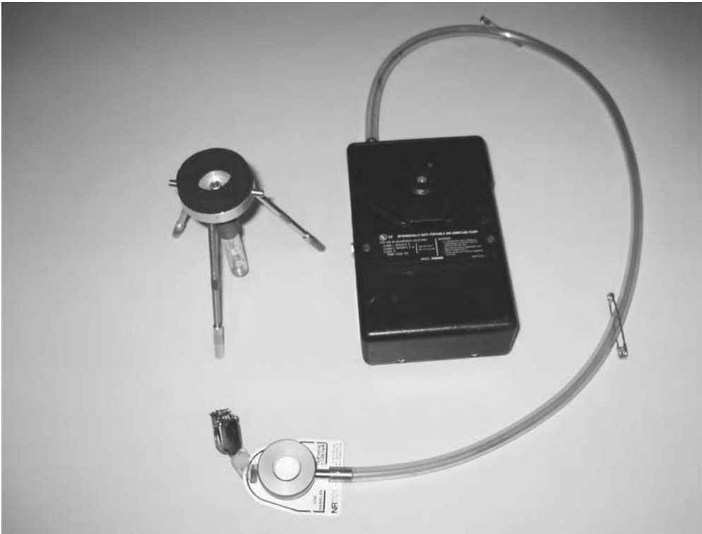
Figure 5.4 Typical personal dust monitor showing pump, sampling head and flowmeter
