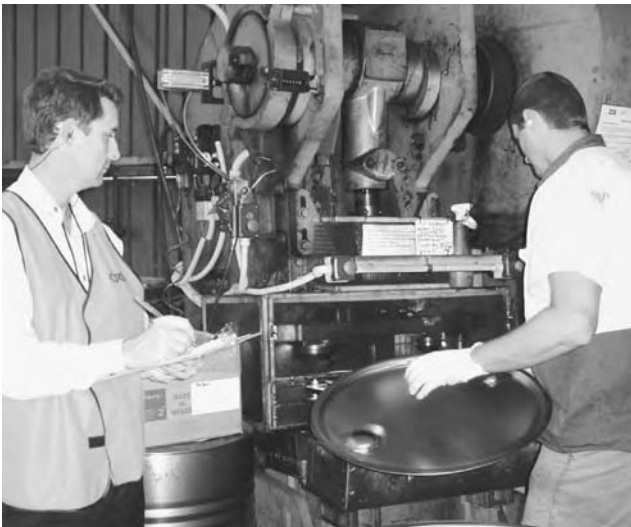
Figure 1.1c Conducting a walkthrough survey in a drum plant; identifying handling processes creating noise
