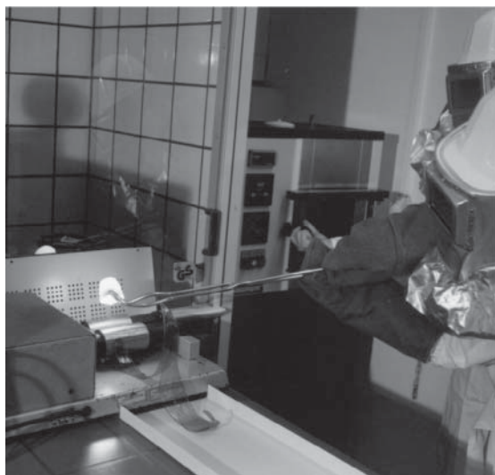
Figure 6.17 Photograph of the of quenched silicate ribbon just coming out between the copper rollers. (Photo: FSU.)
