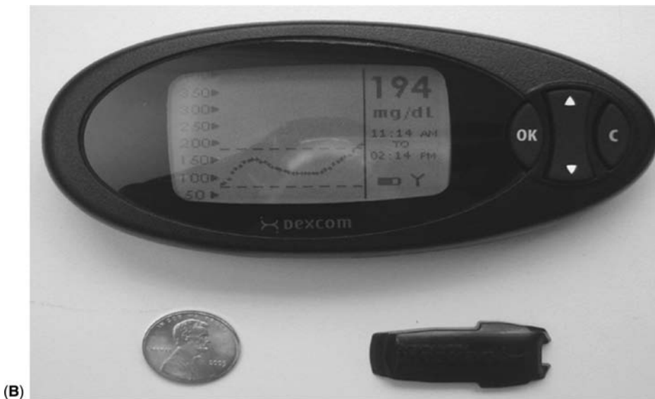
FIGURE 2B DexCom STS Continuous Glucose Monitor displaying glucose measurement (194 mg/dL) on y-axis and time (min) on x-axis. Data from patient-worn sensor/transceiver ( lower right ) is transmitted wirelessly to hand-held monitor with flat-panel display. Monitor is able to display 1, 3, and 9-hour trend data.
