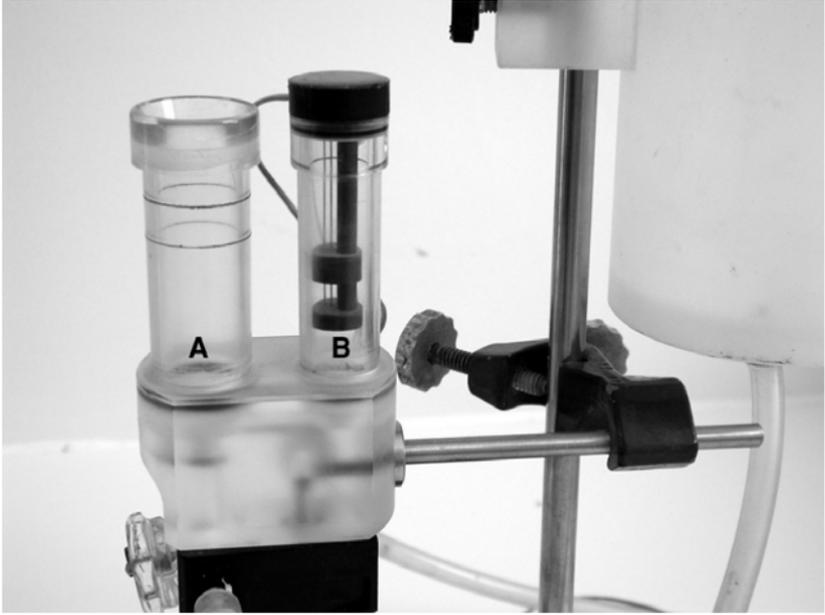
Fig. 2. A water displacement plethysmometer.
