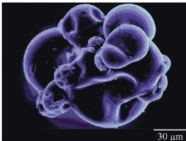
Fig. 10.7 Picture of an agglomerated particle produced by FSD. Reproduced with permission from Hovione FarmaCiencia SA
