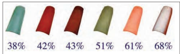
Plate 13 Cool coloured clay tiles and their solar reflectance values
