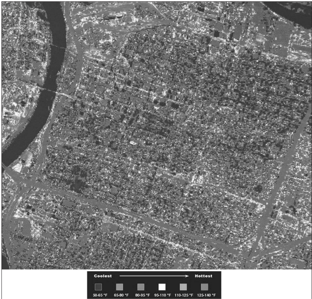
Figure 1.11 Thermal image of downtown Sacramento, California, on 29 June 1998 at noon, derived from a flyover in a Lear jet by NASA's ATLAS program (see Plate 2 for a colour version)
