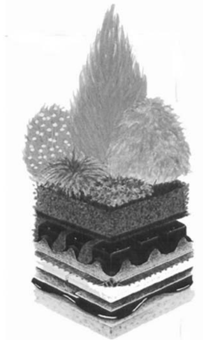
Figure 7.13 Layers of an extensive (left) and an intensive (right) garden roofing system
