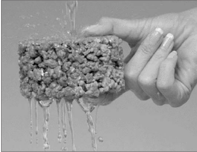
Figure 9.13 Pervious concrete allows water through to the soil underneath
