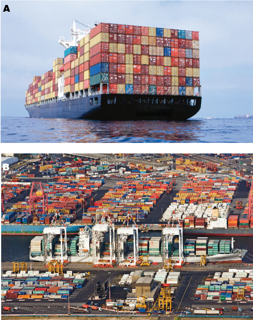
FIGURE 3-5 Containerization. Approximately 90 percent of non-bulk cargo worldwide moves by containers stacked on transport ships. More than 20 million such containers make over 200 million voyages per year; some ships can carry more than 14,500 units. The speed, efficiency, and convenience of this form of transport enable cargoes to be delivered directly from the ship to their destination with minimum delay at the dockside. In consequence, it has become totally impractical to make routine inspections, either at the port of arrival or at the point where the container is finally opened.
